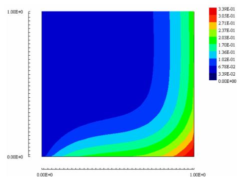
Figure 4. Dimensionless temperature field for Re = 10 and Gr = 0.
