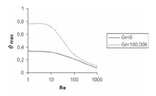
**Figure 3** . Maximum dimensionless temperature as a function of Reynolds number for Gr=0 and  $Gr=1\times10^5$ .
