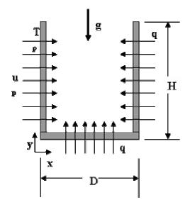
Figure 1. Coordinate system and thermal boundary conditions of the open cavity.
