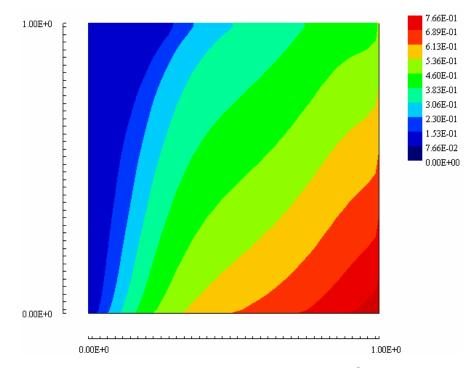
Figure 5. Dimensionless temperature field for Re=10 and Gr=1x10<sup>5</sup>.
