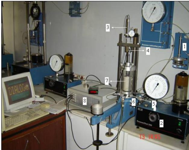
**Figure 2.** Photograph of test apparatus. 1-Volume change transducer, 2-Constant pressure supplier, 3-Displacement transducer (LVDT), 4-Load cell, 5-Pore pressure transducer, 6-Cell pressure transducer, 7-Soil specimen, 8-Data logger.
