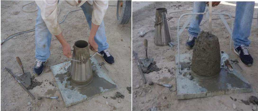
Figure 5. Workability test of studied concrete.
