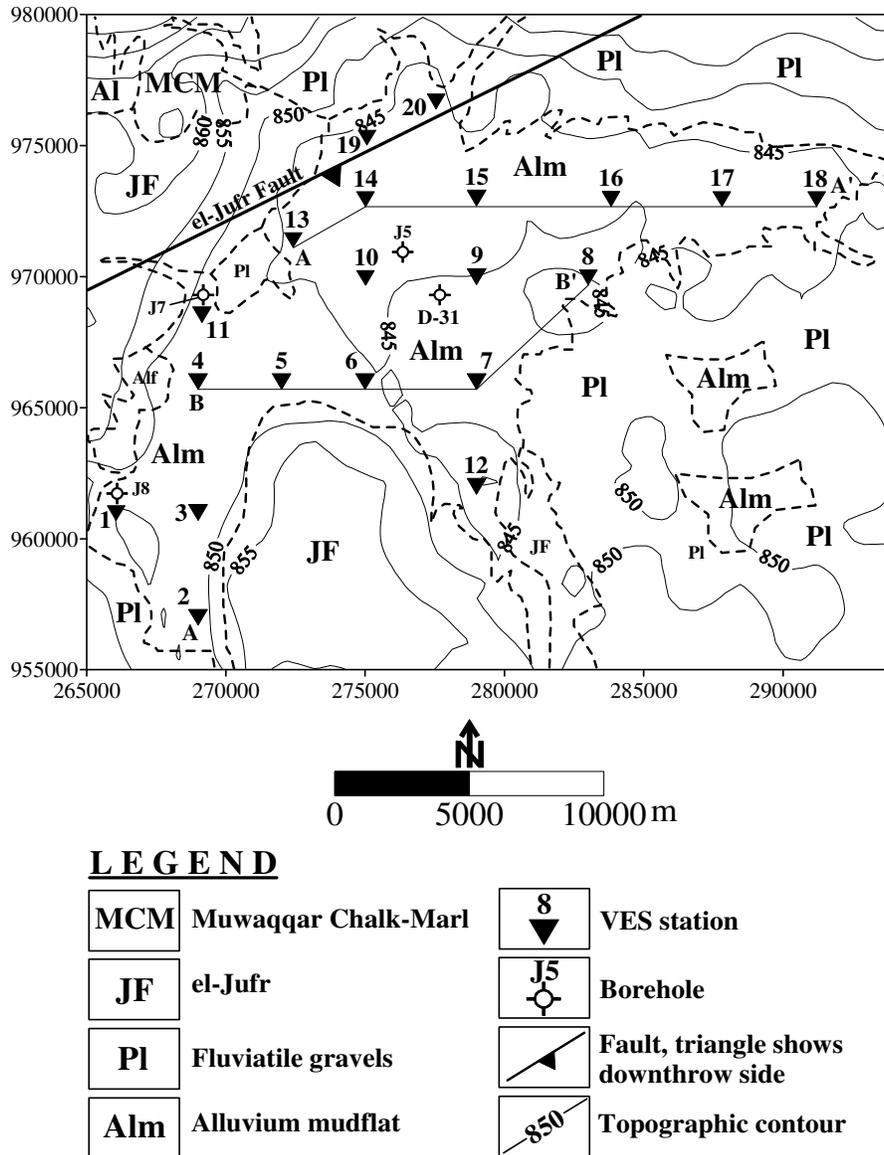
**Figure 2.** Location of VES sites (black triangle) in relation to geology. Also, shown is the location of two profile lines A-A' and B-B' and four boreholes. The elevation contours are in meters. Palestine grid are used.
