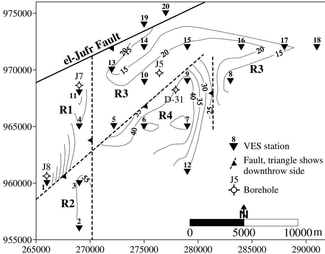
Figure 7. Isopach contour map of the quaternary sediments in relation to inferred structures.
