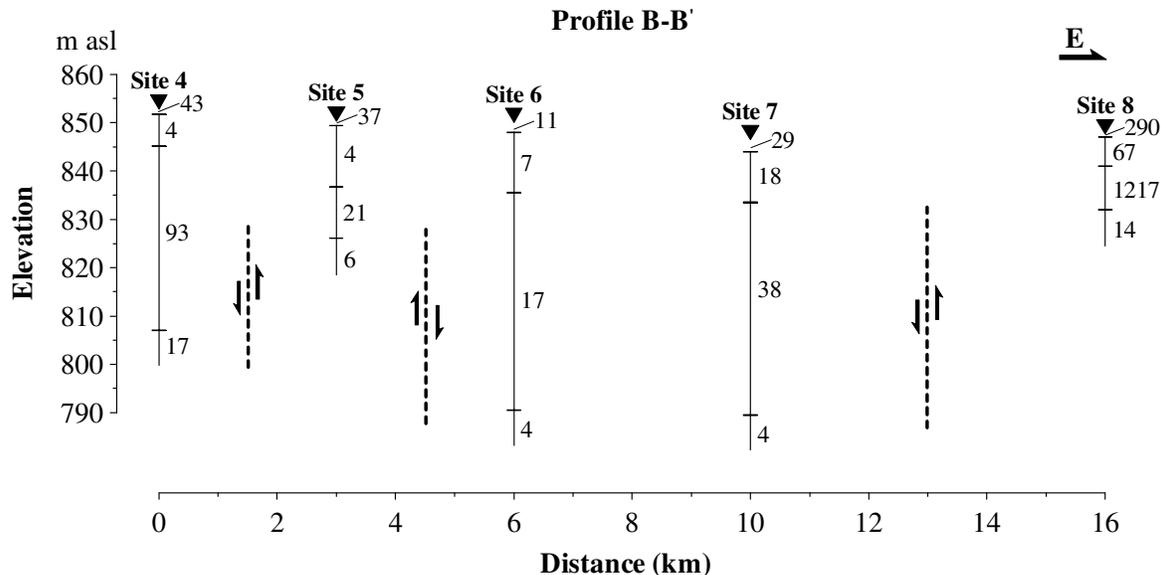
**Figure 6.** Composite geoelectrical cross section inferred from VES data along B-B' (Figure 2: For profile location). Resistivities are in ohm-m.
