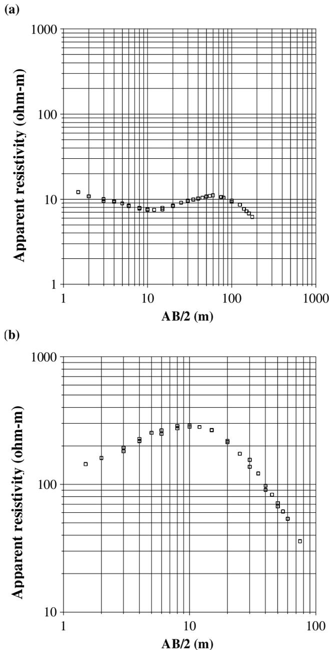
Figure 4. Typical field sounding curves.
