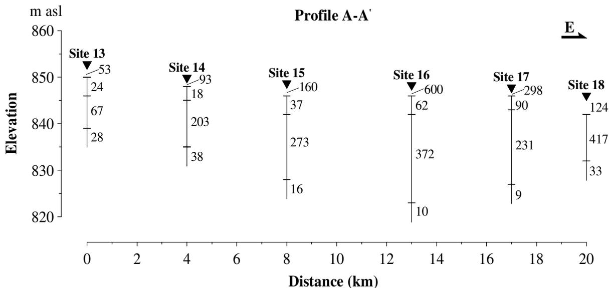
**Figure 5.** Composite geoelectrical cross section inferred from VES data along A-A' (see Fig. 2 for profile location). Resistivities are in ohm-m.
