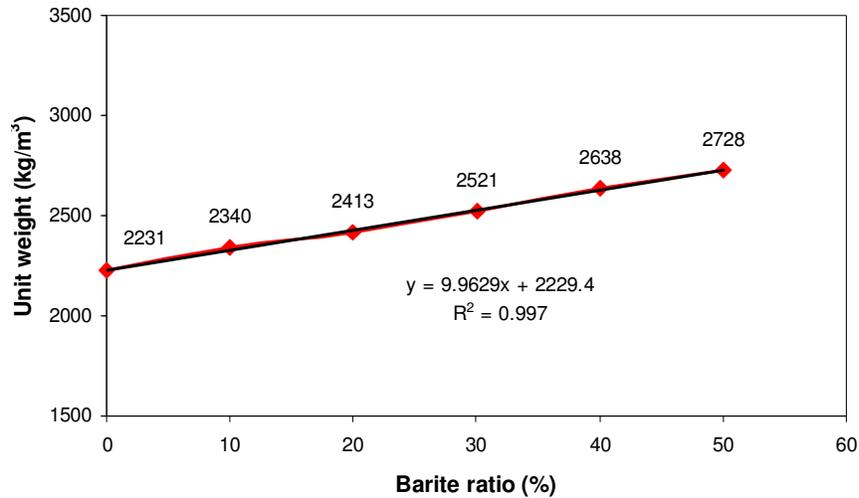
Figure 3. Graph showing change of barite ratio and unit volume weight .
