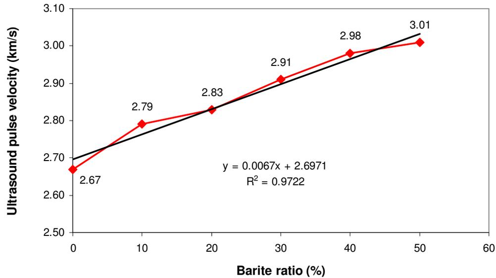
**Figure 5.** Graph showing change of barite ratio in concrete and ultrasonic pulse velocity.
