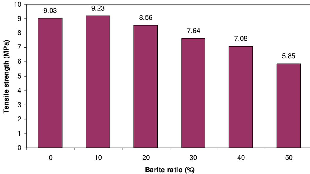
Figure 9. Graph showing change of barite ratio in concrete and tensile strength.
