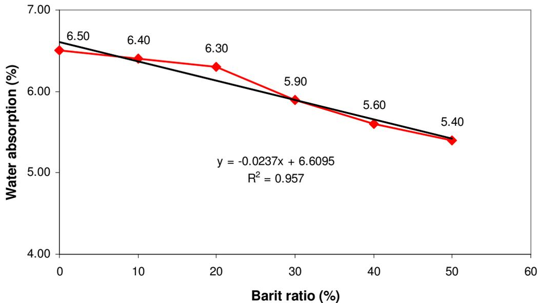
Figure 4. Graph showing water absorption percentage of concrete according to change of barite ratio.
