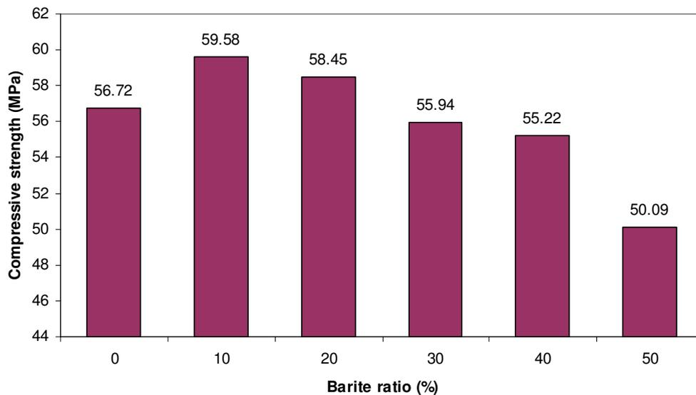
**Figure 8.** Graph showing change of barite ratio in concrete and compressive strength.
