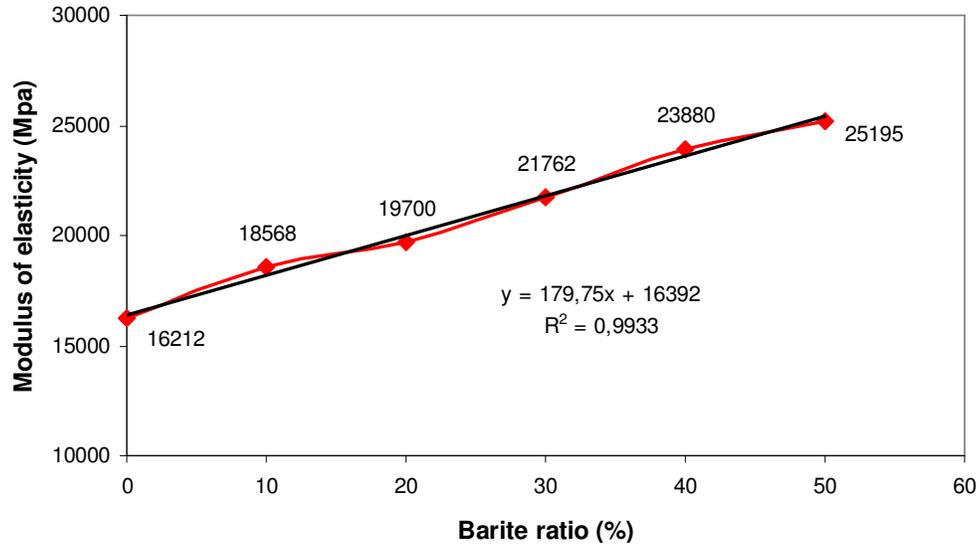
**Figure 7.** Graph showing change of modulus of elasticity in concrete according to barite ratio.
