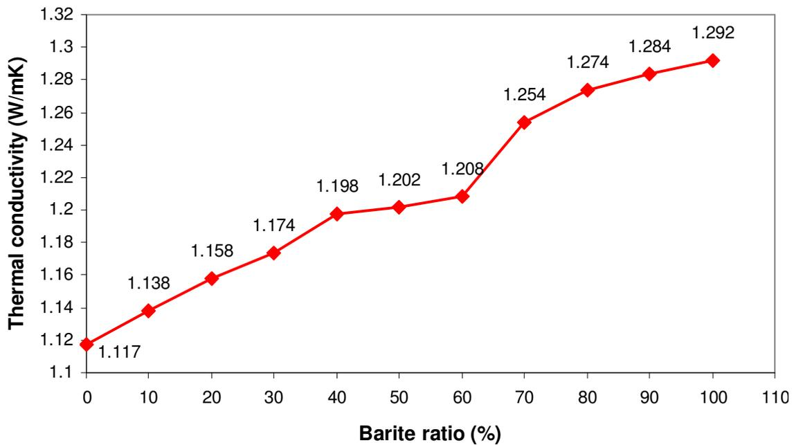
Figure 10. Graph showing change of barite ratio in concrete and thermal conductivity.
