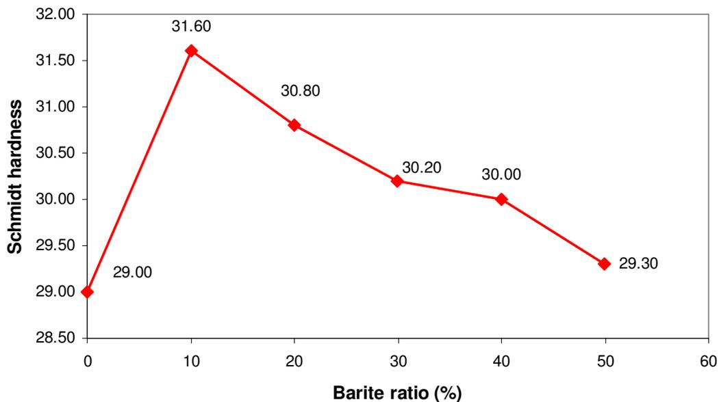
**Figure 6.** Graph showing change of barite ratio in concrete and Schmidt hardness.
