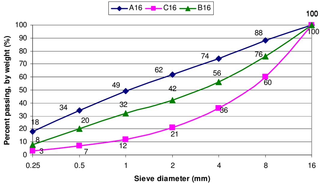
Figure 1. Granulometry curve of aggregates used in the experiments.
