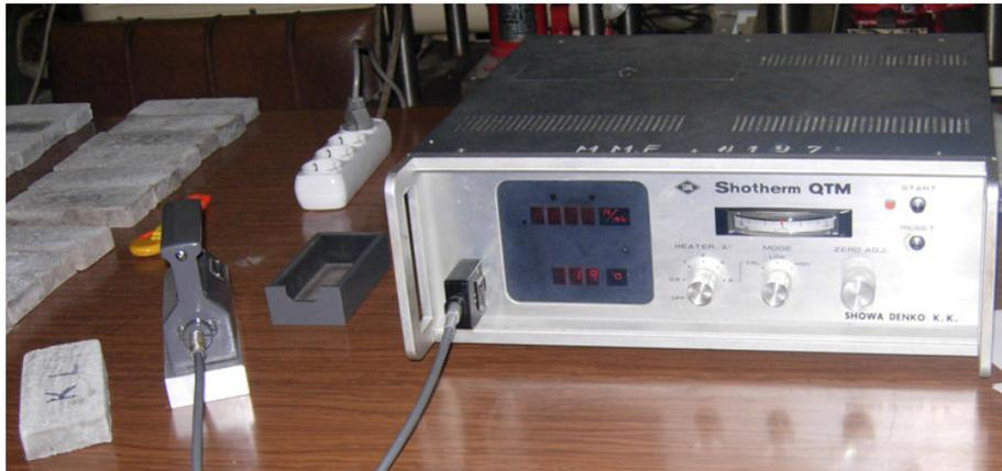
**Figure 2.** Thermal conductivity coefficient measurement device with hot wire method.
