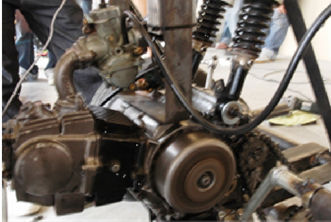
Figure 1. Standard 115cc motorcycle engine salvaged from scrapped yard.
