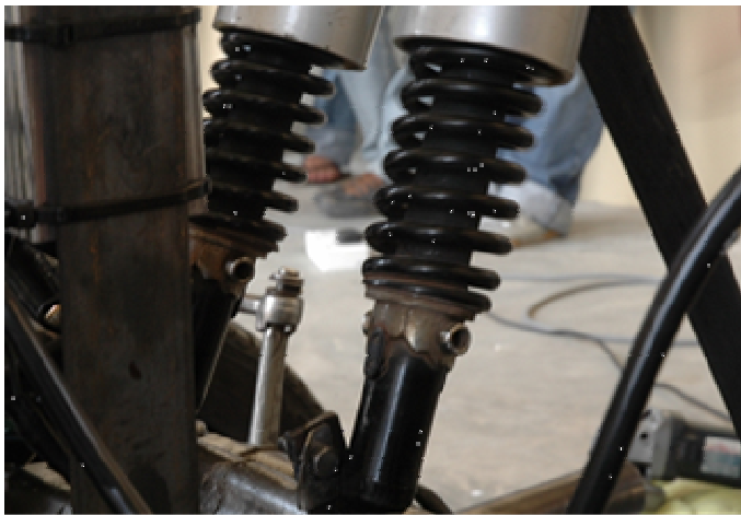
Figure 2. Engine shock absorber from typical motorcycle suspension system.
