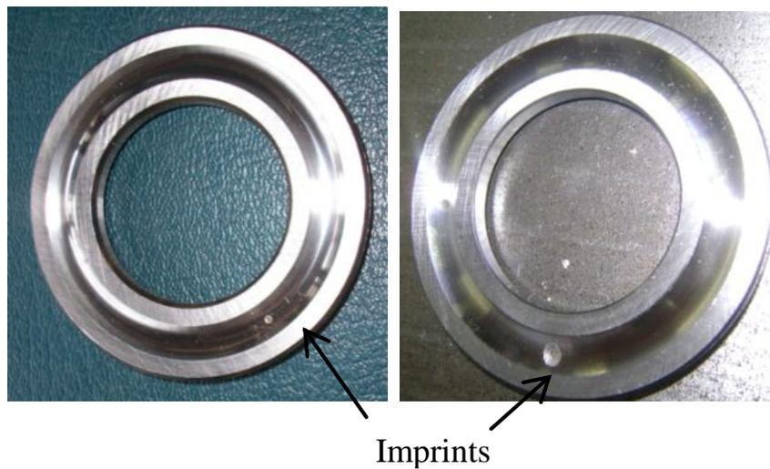
**Figure 4.** Spalling defect on a thrust ball bearing.
