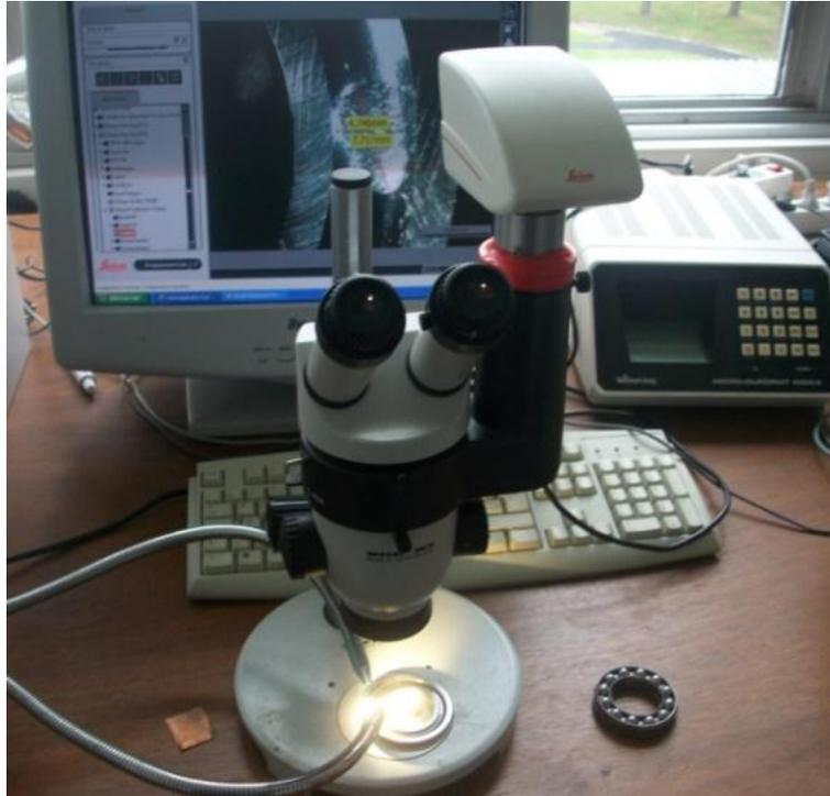
Figure 5. Measurement of the spalling fault size.
