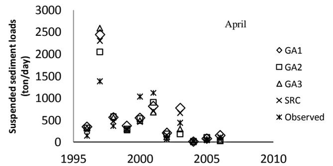
**Figure 8.** The scatter plot of the discharge against the observed suspended sediment load and the estimated suspended sediment by GA models of Nodeh station during test period in April.
