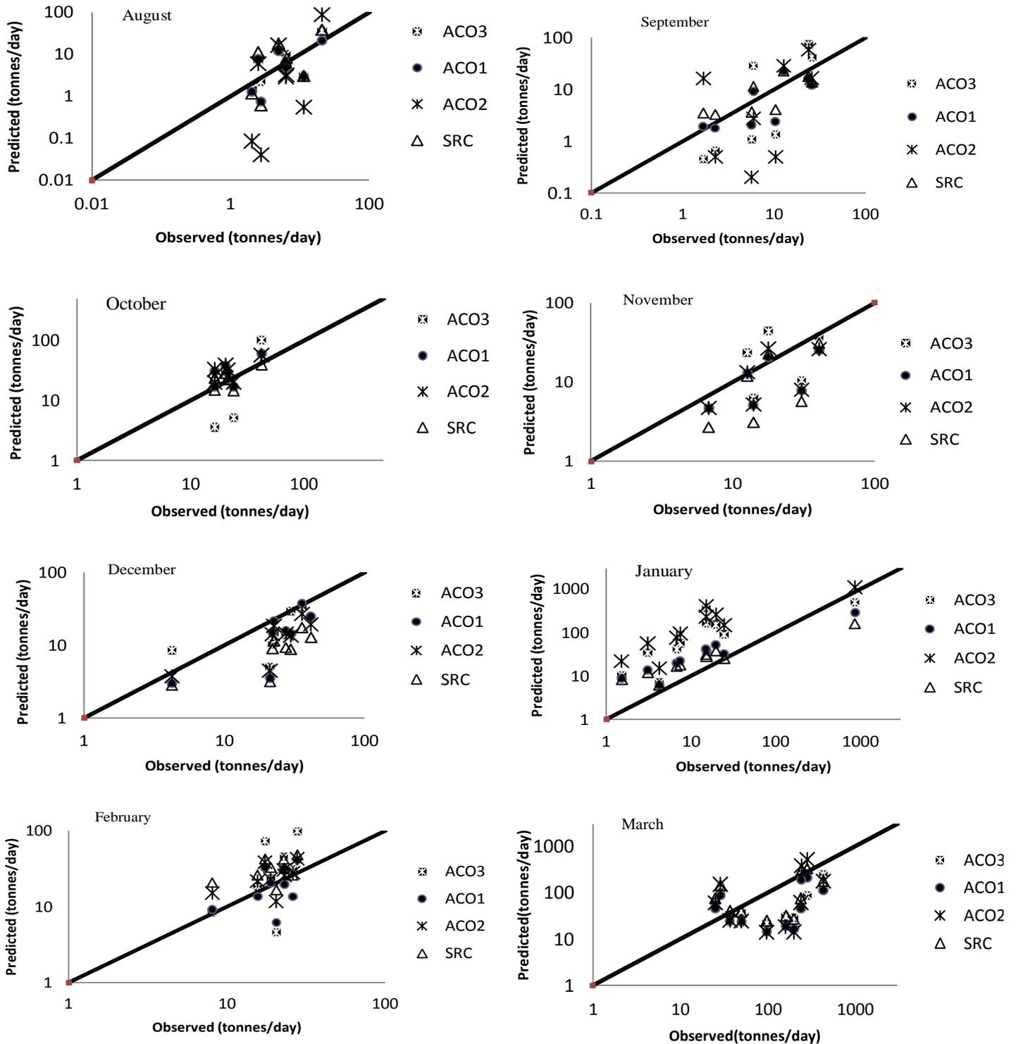
Figure 11. Scatter plot for observed and predicted suspended sediment for test period for various model of ACO.
