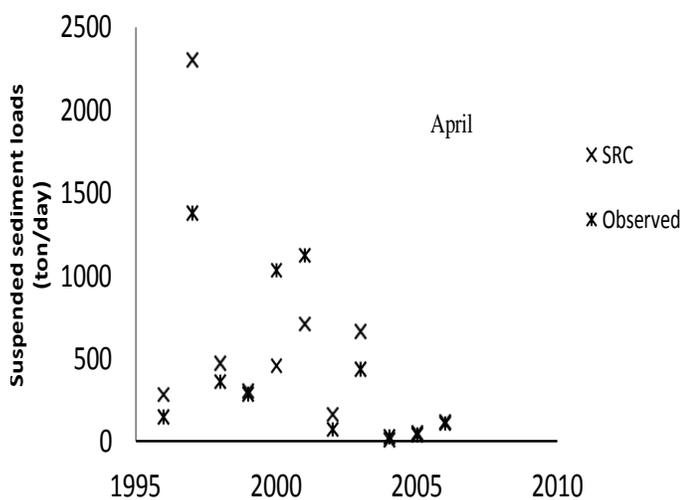
**Figure 7.** The scatter plot of the discharge against the observed suspended sediment load and the estimated suspended sediment by SRC of Nodeh station during test period in April.
