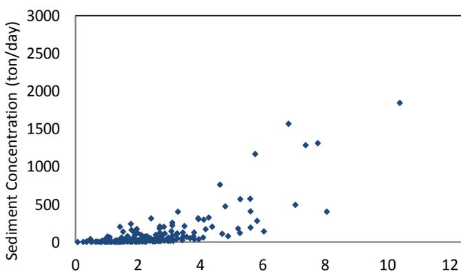
**Figure 5.** Suspended sediment load–discharge scatter diagram for all data for the Nodeh station.
