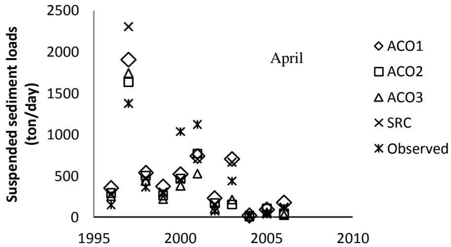
**Figure 10.** The scatter plot of the discharge against the observed suspended sediment load and the estimated suspended sediment by ACO models of Nodeh station during test period in April.
