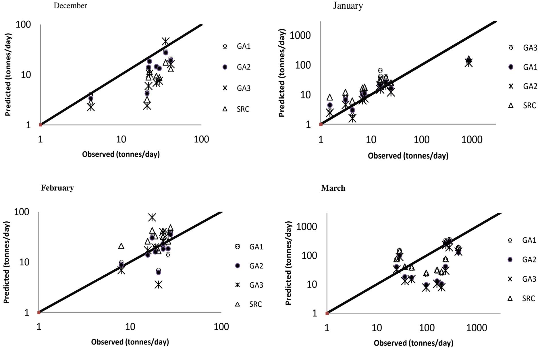
Figure 9. Scatter plot for observed and predicted suspended sediment for test period for various model of GA.
