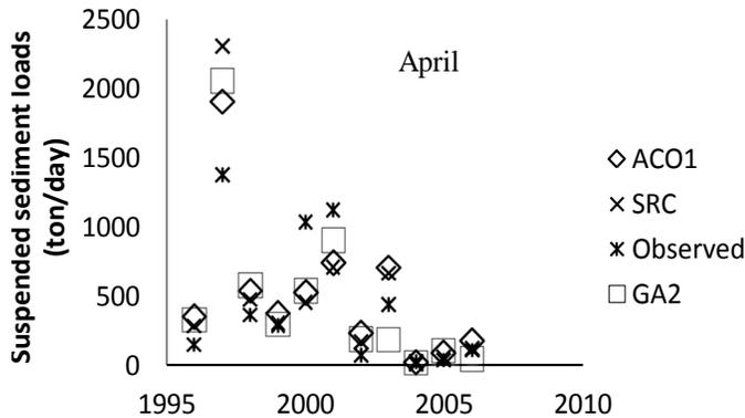
**Figure 12.** The scatter plot of the discharge against the observed suspended sediment load and the estimated suspended sediment by the best ACO, best GA and SRC models of Nodeh station during test period in April.
