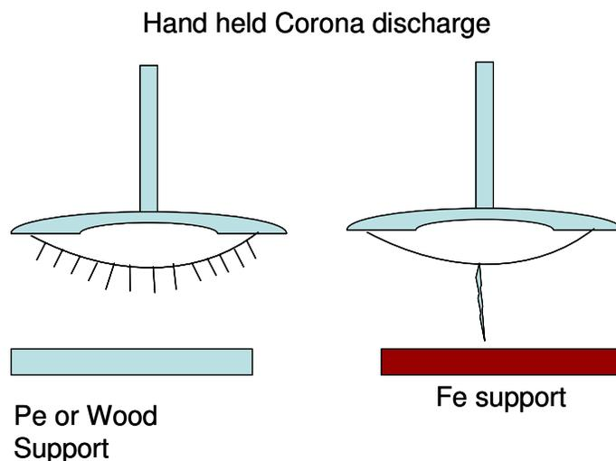
**Figure 3.** Nature of glow discharge and electrical sparc on different support media.
