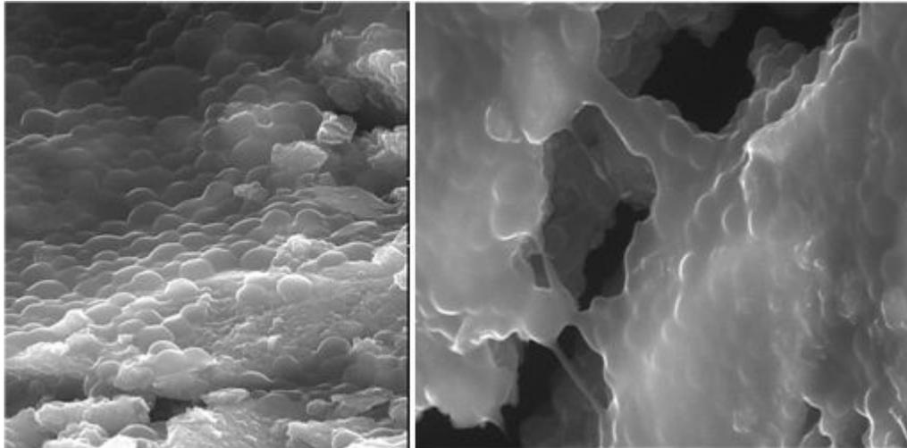
**Figure 1.** Scanning electron micrographs showing film formation over the surface of silica particles.
