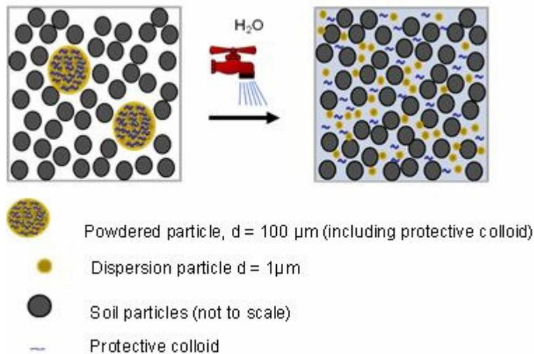
**Figure 2.** Upon addition of water, polymer powders were redispersed into their original dispersion particles.
