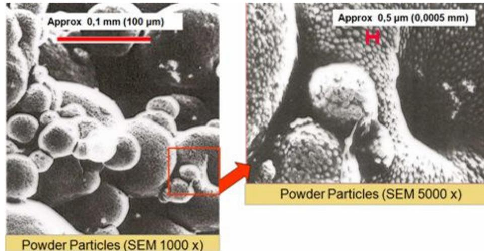
**Figure 5.** Scanning electron microscopy on polymer dispersible powders reveal their structure.
