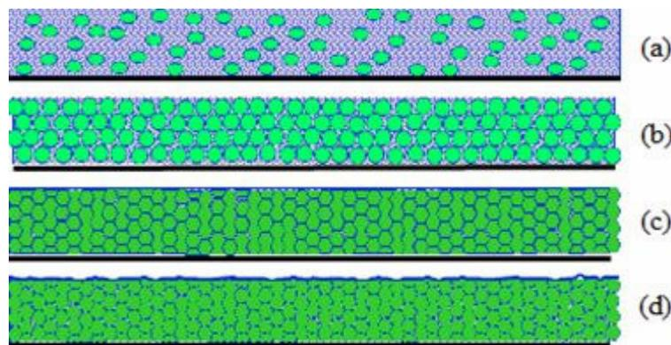
**Figure 4.** a) Dispersion with individual polymer particle; b) Evaporation: Particles converge; c) At the end of evaporation process: Deformation of particles; d) Formation of a homogeneous film by interdiffusion of the particles.
