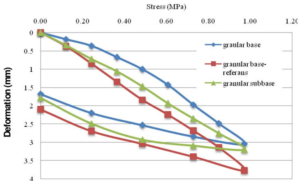
Figure 8. Plate loading tests conducted on base and subbase layers of the road.
