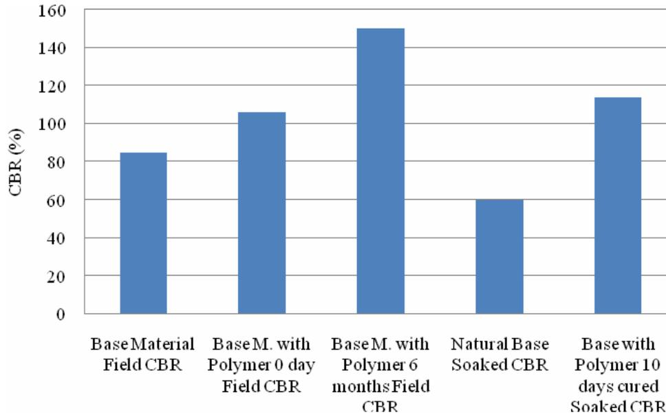
**Figure 11.** Field CBR and laboratory soaked CBR results.
