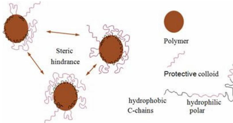
**Figure 3.** Independent polymer solids in the dispersed phase.
