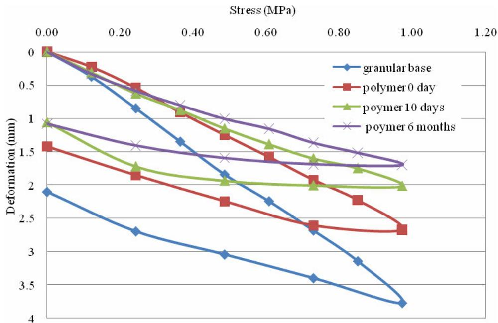
**Figure 9.** Time-series comparison of plate loading tests conducted on base material and base layer with polymer additive.**Table 3.** Summary of plate loading tests and relative density of base layers with polymer additive.
