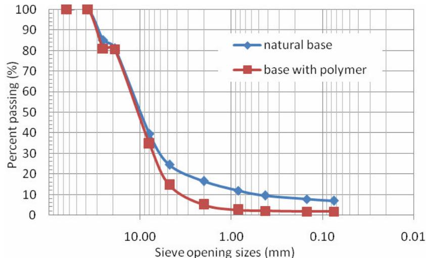
Figure 7. Grain size analysis of base material and base material with polymer.
