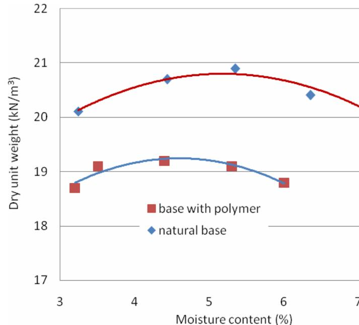
**Figure 6.** Modified proctor tests.
