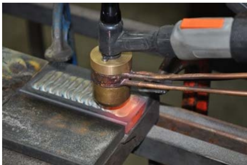
Figure 4. Photo of the device after the operation, configuration concentric with 8 holes, adapted to the torch GTAW/PTA with deposition automatic.
