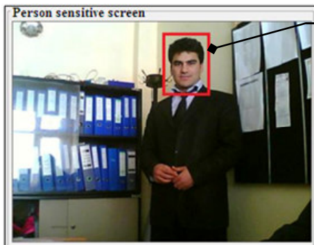
Figure 7. The identification of the facial area by skin color algorithms and geometric techniques.
