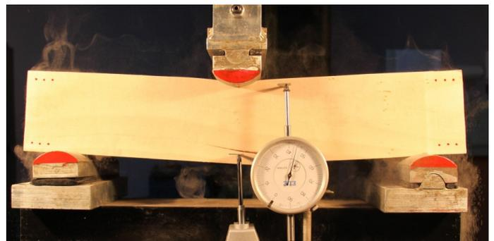
Figure 15. The failure of the 3rd testing sample under load.
