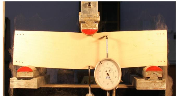
Figure 14. The failure of the 2nd testing sample under load
