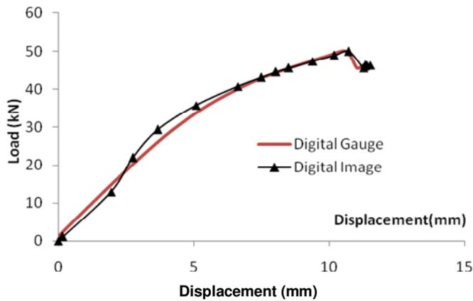
Figure 10. The load-displacement relationship of digital image and the comparator of 2nd sample.
