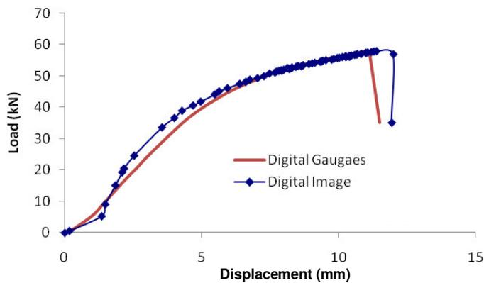
Figure 11. The load-displacement relationship of digital image and the comparator of 3rd sample
