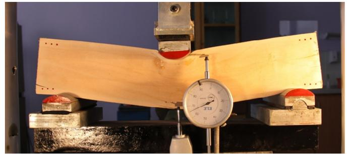
Figure 13. The failure of the 1st testing sample under load.
