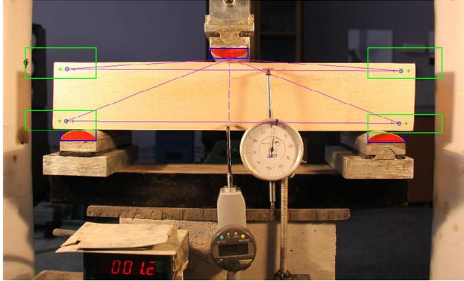
Figure 5. The calculation of the top and bottom displacement values of the sample.
