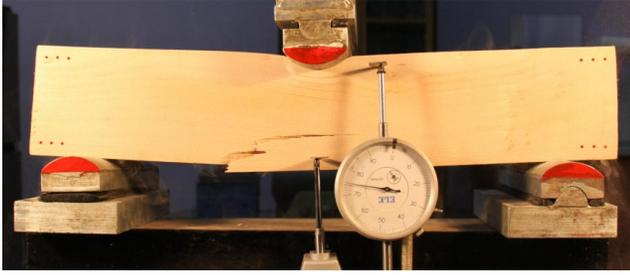
**Figure 16.** The failure of the 4th testing sample under load.
