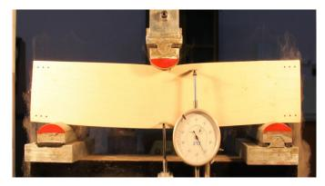
Figure 14. The failure of the 2nd testing sample under load
