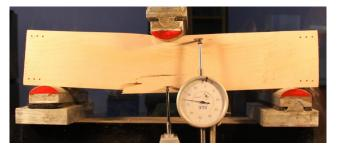
Figure 16. The failure of the 4th testing sample under load.
