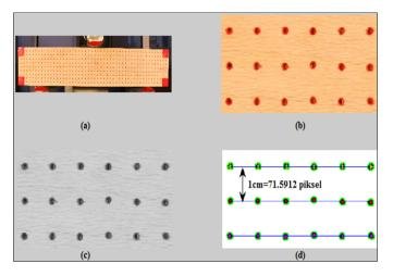
Figure 6. The conversion of 1cm into pixel value.
