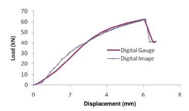
**Figure 12.** The load-displacement relationship of digital image and the comparator of 4th sample.
