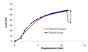
Figure 11. The load-displacement relationship of digital image and the comparator of 3rd sample
