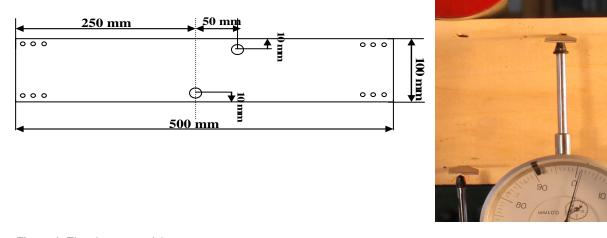
Figure 8. The placement of the comparators.
