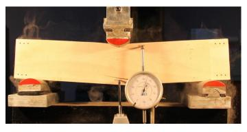
Figure 15. The failure of the 3rd testing sample under load.
