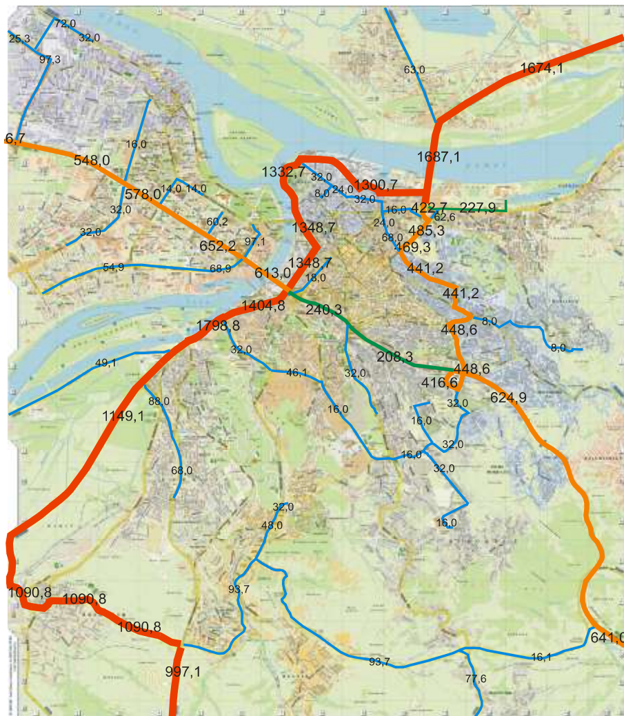
Figure 6. Oil and oil derivatives flow on city roads (in thousands of liters).
