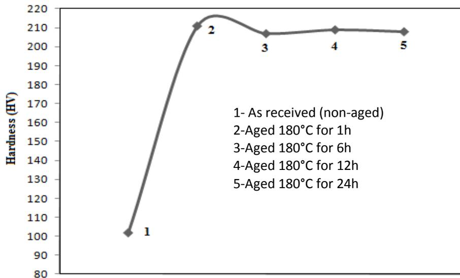
**Figure 1.** Hardness values of the As-received and aged samples.
