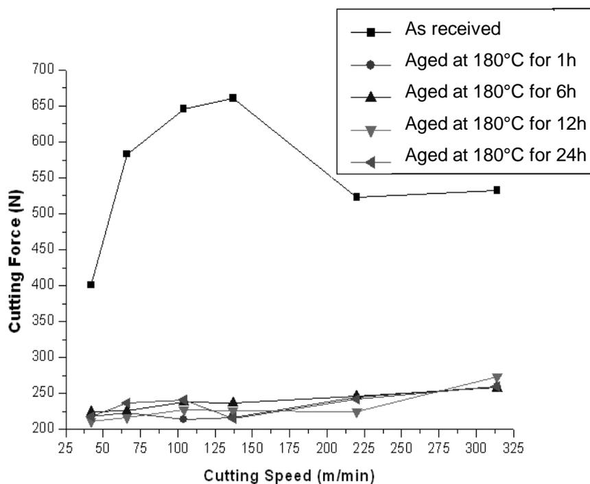
**Figure 2.** The effect of different conditions and cutting speeds on cutting forces of 7075 Al alloy.
