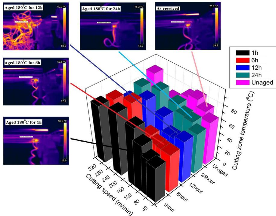
**Figure 5.** The effects of aging parameters on cutting heat treatment at the cutting speed of 66 m/min.
