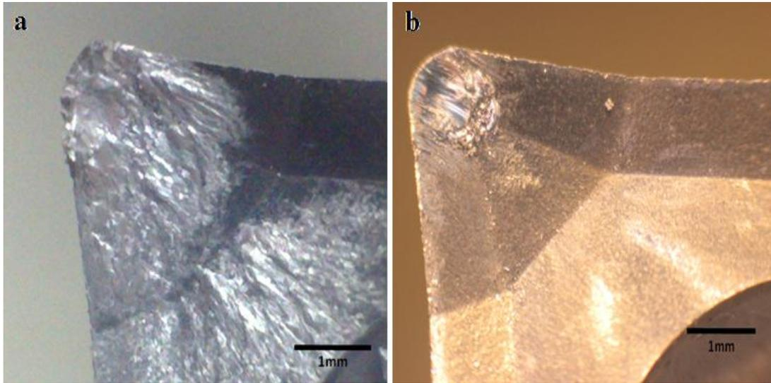
**Figure 3.** The effect of BUE (built up edge) on cutting tools a- As-Received and b- Aged at 180°C for 1 h.
