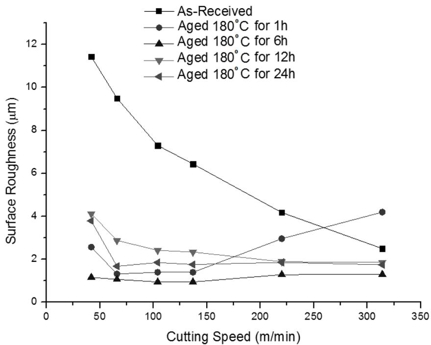
**Figure 4.** The influence of cutting speeds and aging time on the machined test sample surface roughness values.
