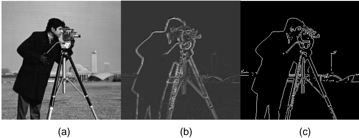
Figure 8. Edge detection on image "Cameraman", (a) original image, (b) the local maximum edge strength (c) edges detection obtained by the proposed technique.
