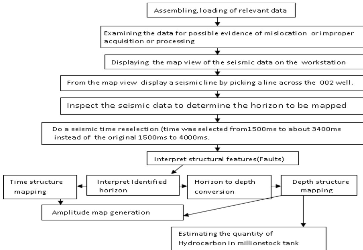
Figure 4. Flow chart of the analytic procedure.
