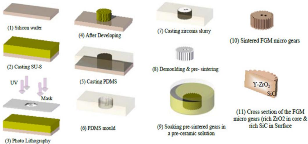
**Figure 3.** Schematic diagram of infiltration process of YSZ/SiC FGM (Hassannin and Jiang, 2010).
