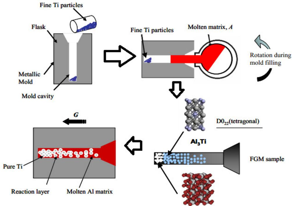
Figure 4. A schematic illustration showing CMPM (Watanabe et al., 2009).
