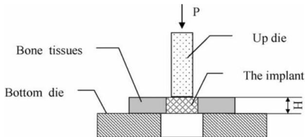
**Figure 1.** Schematic diagram for testing the shear bonding strength between the tissues and the implant ( $P$ : extruding force,  $H$ : thickness of implant) (Chu et al., 2006).
