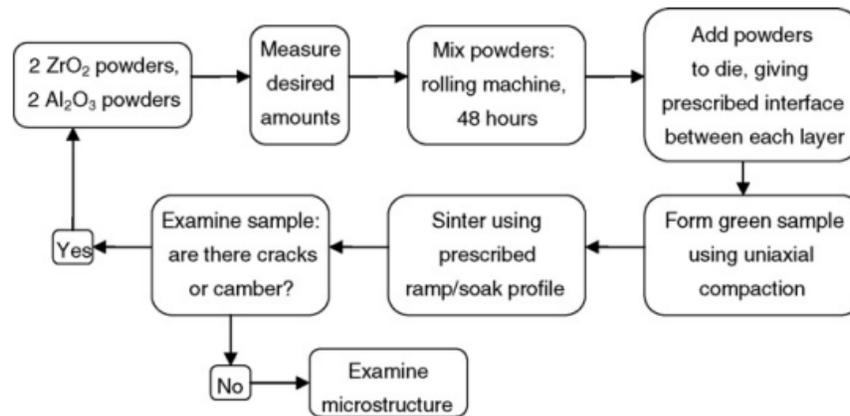
**Figure 2.** Flow chart detailing the manufacturing process of  $\text{Al}_2\text{O}_3/\text{ZrO}_2$  FGM used in Sun et al. (2008).
