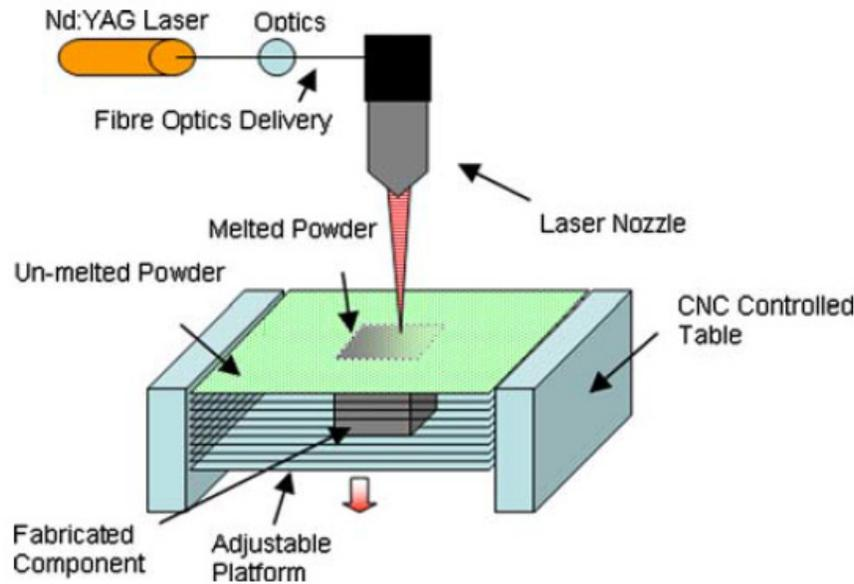
**Figure 5.** Experimental setup for laser assisted processing using Nd:YAG laser power source (Mumtaz and Hopkinson, 2007).
