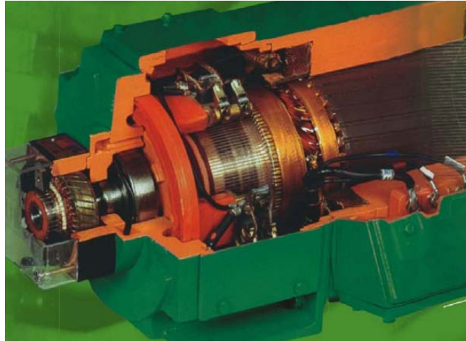
Figure 1. Cutaway description of a DC motor (INO, 2010).
