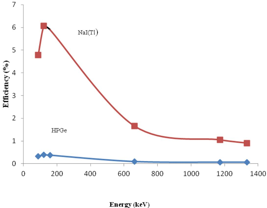
**Figure 3.** Efficiency of HPGe detector and NaI (TI) detector as function of energy.
