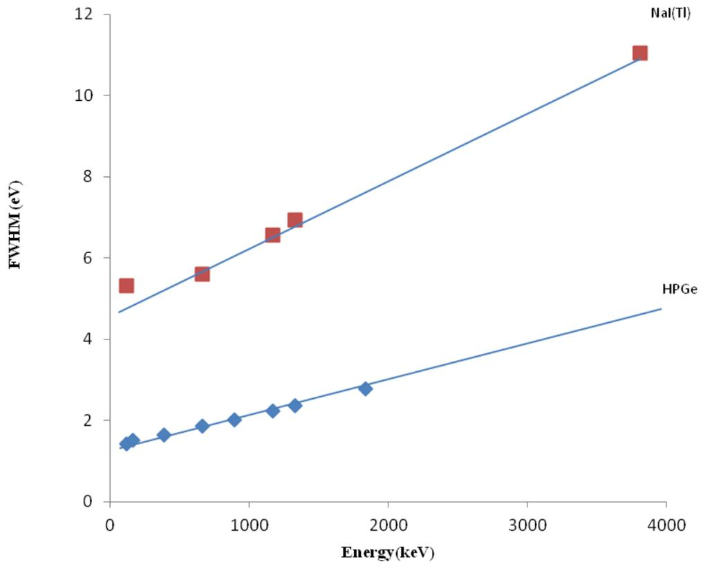
Figure 2. Resolution of HPGe detector and NaI (Tl) detector as function of energy.
