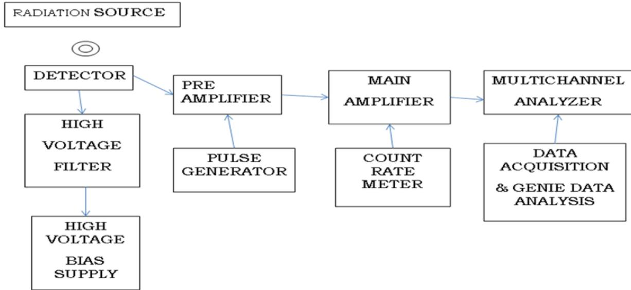
Figure 1. Block diagram of the experimental setup.
