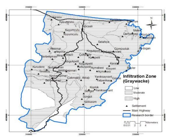
Figure 6. Infiltration zones of the Graywackes in the research area.
