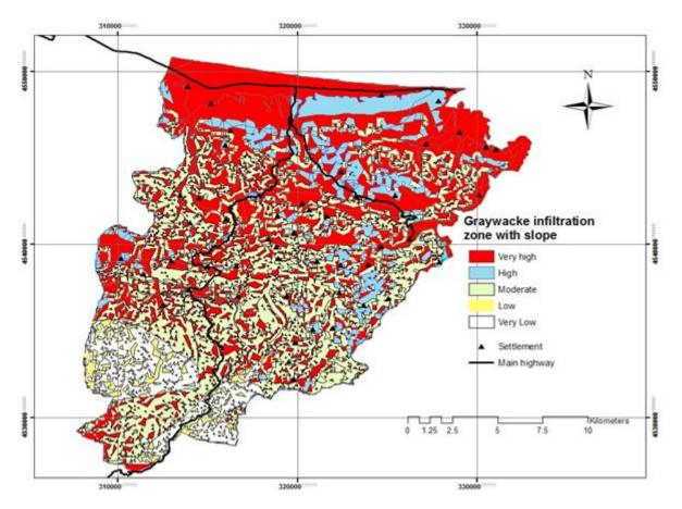
Figure 7. Graywacke permeability values in the research area (slope and rock permeability values).
