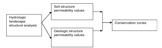
Figure 3. The method of pointing infiltration zones with hydrologic landscape analysis (Buuren 1994, Şahin 1996).
