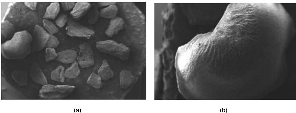
**Figure 2.** Grinded slag waste particle for 200  $\mu\text{m}$ : (a) SEM picture of 9x mag and (b) Scaled up picture of a particle (33x mag).
