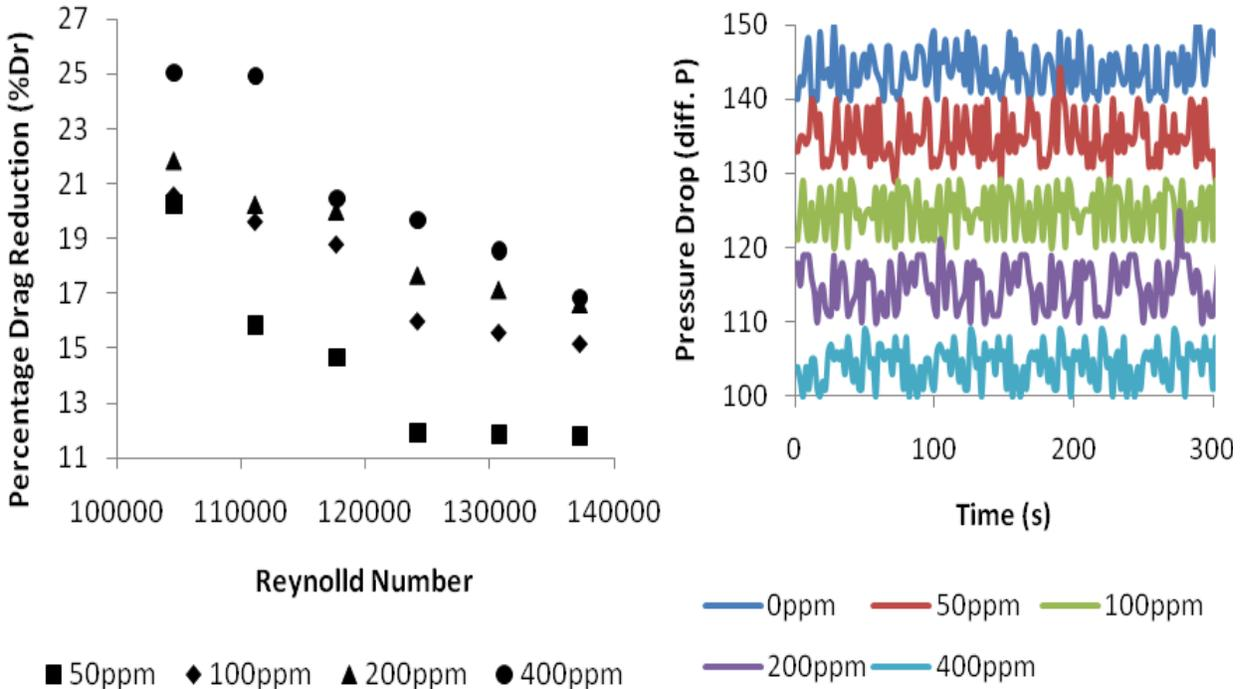
**Figure 3.** Effect of particle concentration in transported fuel on Dr% with different Re in 0.0381 n D.I and 2.0 m pipe length and pressure drop analysis for Re = 105000.
