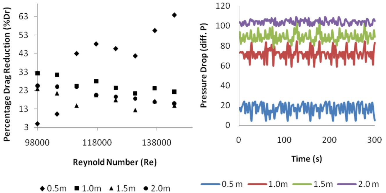
Figure 7. Effect of pipe length in 400 ppm addition concentration flowing in fuel with pipe diameter 0.0381 m D.I and pressure drop data for Re = 139000.
