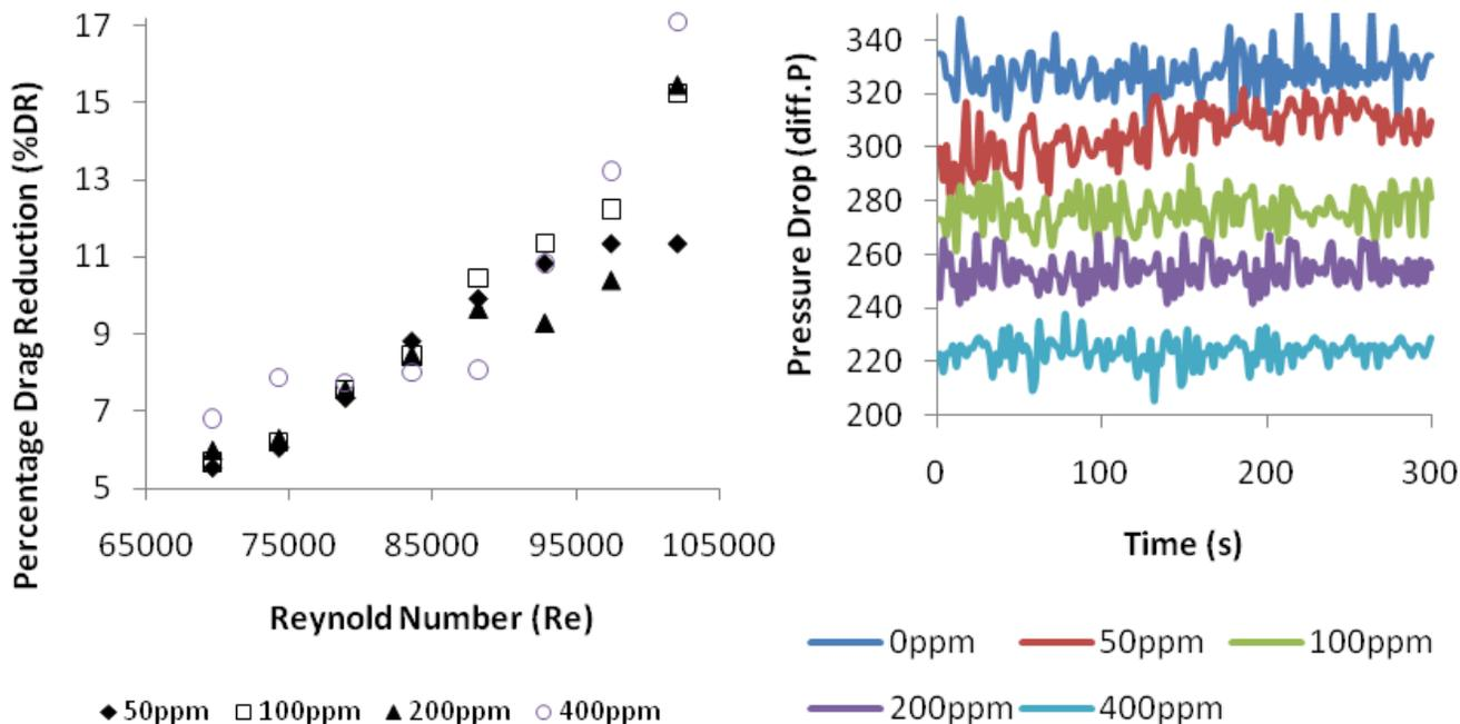
Figure 4. Effect of particle concentration in transported water on Dr% with different Re in 0.0381 n D.I and 2.0 m pipe length and pressure drop analysis for Re = 105000.
