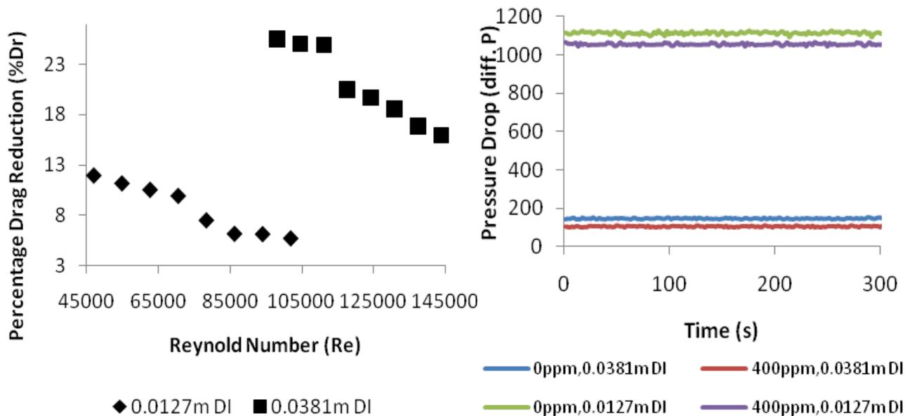
Figure 5. Effect of pipe diameter flowing through 2 m pipe length in fuel and 400 ppm concentration addition and pressure drop data for pipe diameter of 0.0127 and 0.0381 m D.I.
