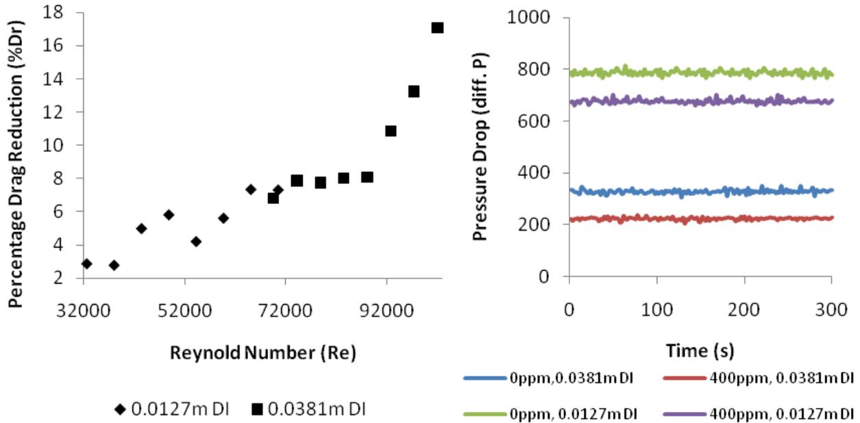
Figure 6. Effect of pipe diameter flowing through 2 m pipe length in water and 400 ppm concentration addition and pressure drop data for pipe diameter of 0.0127 and 0.0381 m D.I.
