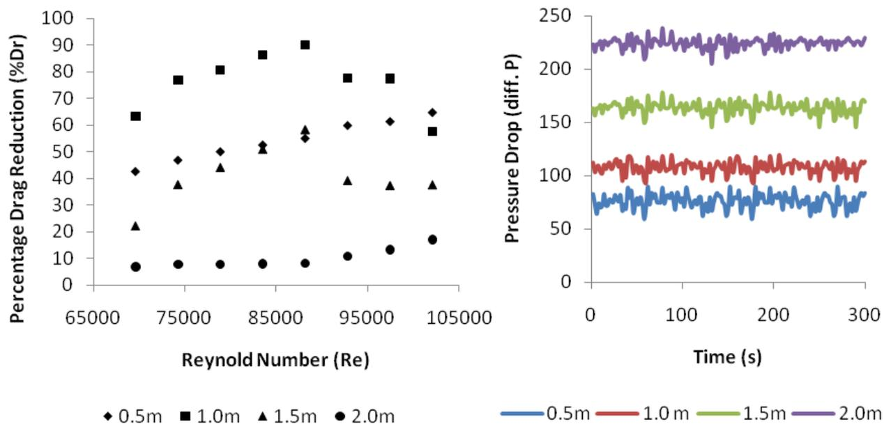
**Figure 8.** Effect of pipe length in 400 ppm additive concentration flowing in water with pipe diameter 0.0381 m D.I and pressure drop data for Re = 100000.
