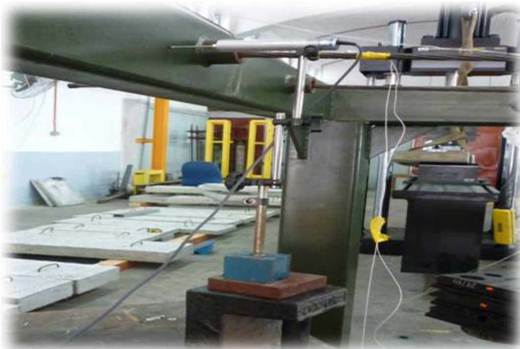
Figure 5. Linear variable differential transformer used on steel frame.
