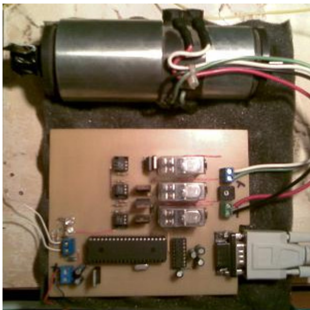
Figure 5. Picture of DC motor, generator and driver.
