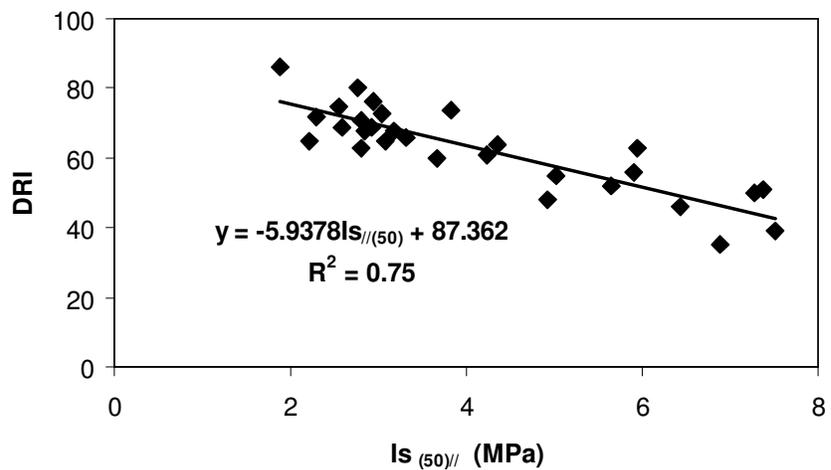
**Figure 10.** DRI of different rock type correlated with axial point load strength index ( $Is_{(50)//}$ ).
