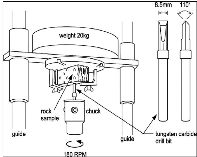
Figure 1. Outline of the Sievers' J miniature drill test (Dahl, 2003).
