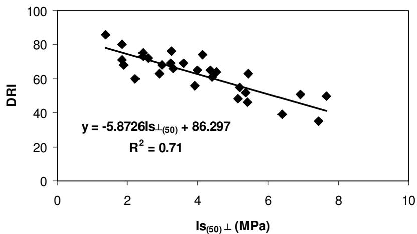
**Figure 9.** DRI of different rock type correlated with diametral point load strength index ( $Is_{(50)\perp}$ ).
