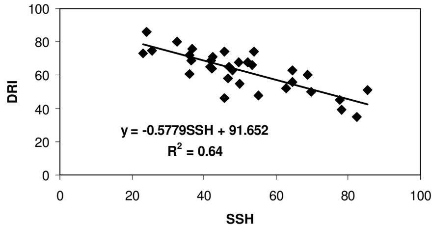
**Figure 8.** DRI of different rock type correlated with shore scleroscope hardness (SSH).
