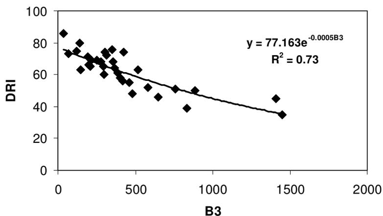
**Figure 4.** Relationship between brittleness (B3) and drilling rate index (DRI).
