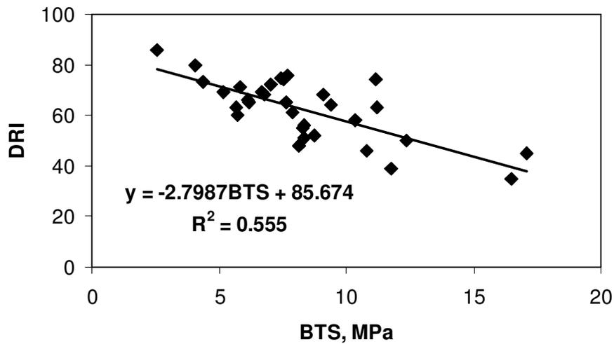
Figure 7. DRI of different rock type correlated with BTS.
