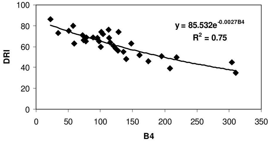
Figure 5. Relationship between brittleness (B4) and drilling rate index (DRI).
