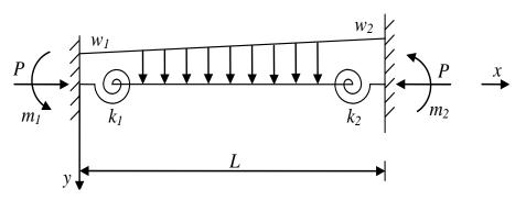
Figure 5. Linear variation of load.
