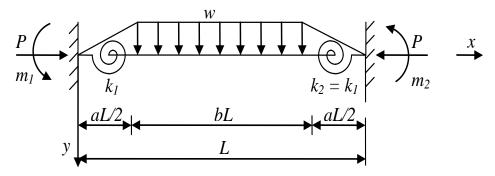
Figure 6. Symmetrical trapezoidal load.
