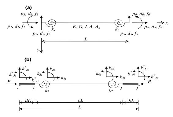
Figure 1. (a) Beam-column member model and (b) Beam-column member model with rigid end sections.
