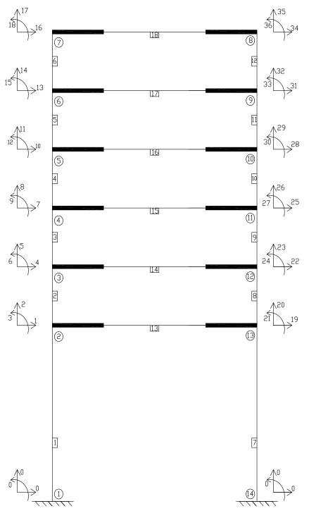
Figure 9. Coding and numbering of the example problem.
