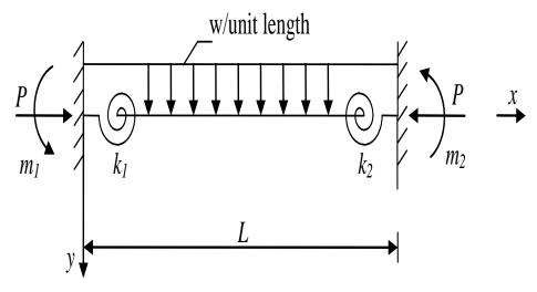
Figure 3. Uniformly distributed load.
