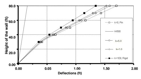
Figure 10. Lateral deflections at each floor level in the example problem with varying spring constants k.
