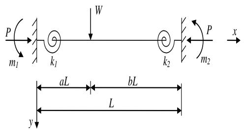
Figure 4. Single-point load.
