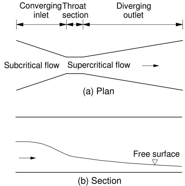
Figure 3. Venturi weir (a) plan; (b) section.
