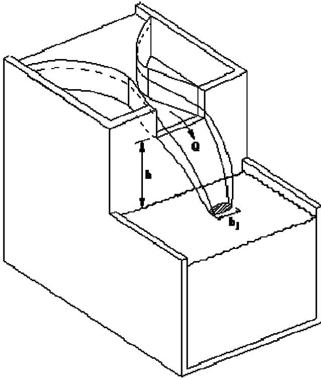
Figure 1. Free overfall jet over a venturi weir.
