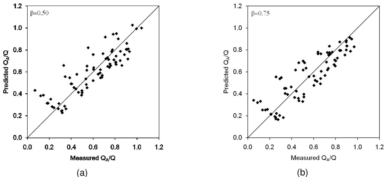
Figure 12. Comparison of measured air-demand ratio values with those calculated from Equations 3 and 4 for (a)  $\beta=0.50$ ; (b)  $\beta=0.75$ .
