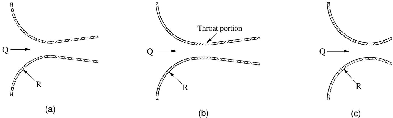
**Figure 6.** Venturi weir types used in the experiments: (a) throatless venturi weir; (b) throated venturi weir; (c) circular venturi weir.
