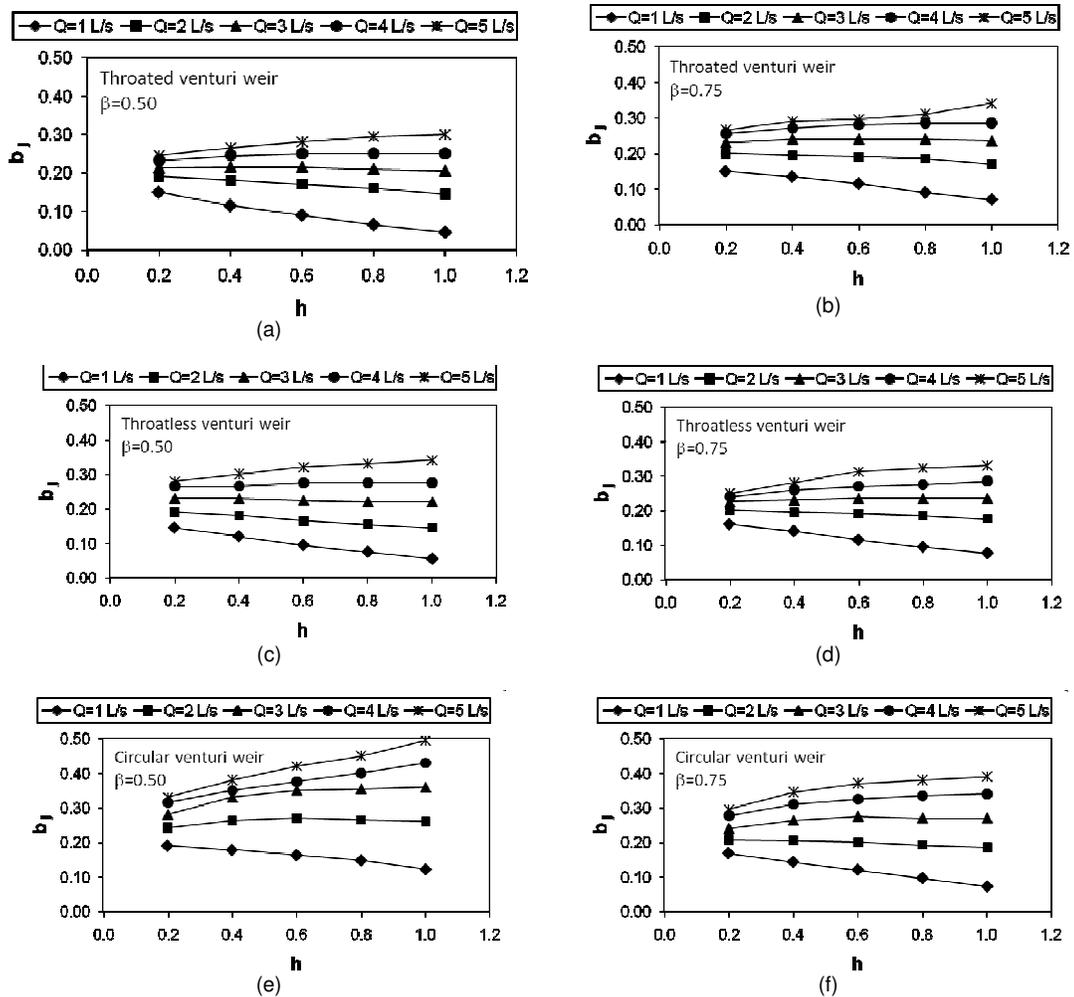
Figure 10. Variation in free overfall jet width at the point of impact with drop height and water discharge for different weir types and constriction ratios.
