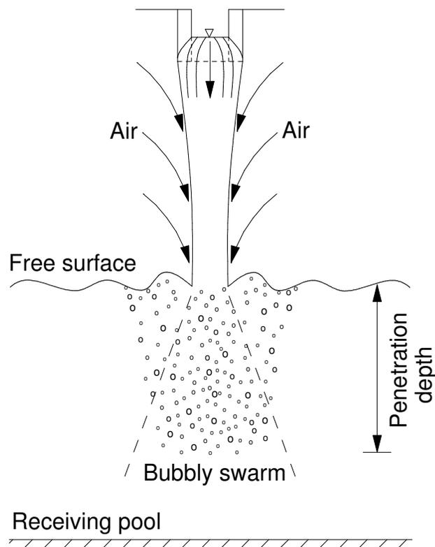
Figure 2. Air entrainment by free overfall jet from a venturi weir.
