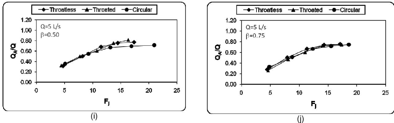
Figure 11. Variation in air-demand ratio with jet Froude number and weir type for different discharges and constriction ratios.
