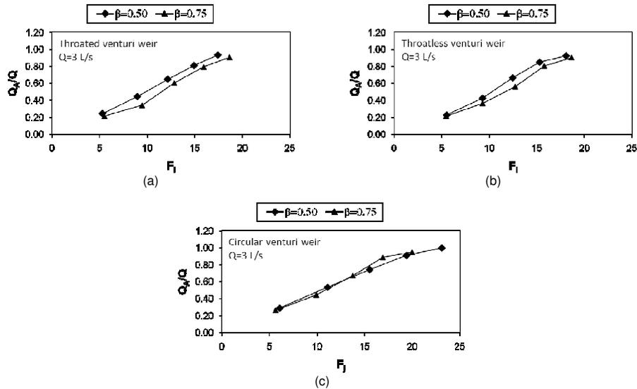
Figure 9. Variation in air-demand ratio with jet Froude number and constriction ratio for different weir types.
