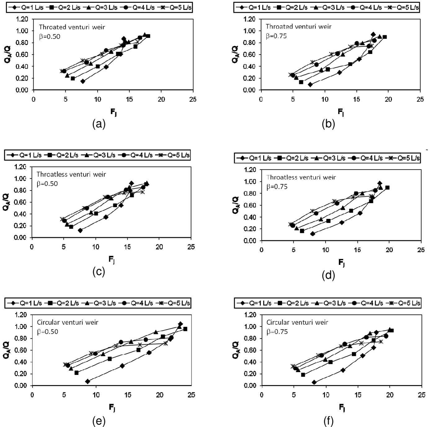
Figure 7. Variation in air–demand ratio with jet Froude number and water discharge for different weir types and constriction ratios.
