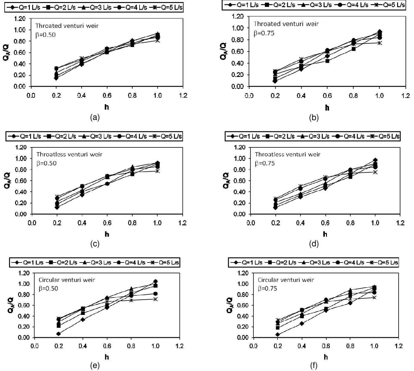
**Figure 8.** Variation in air–demand ratio with drop height and water discharge for different weir types and constriction ratios.
