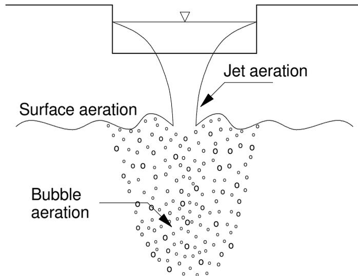
Figure 4. Weir aeration mechanisms (Mueller et al., 2002).
