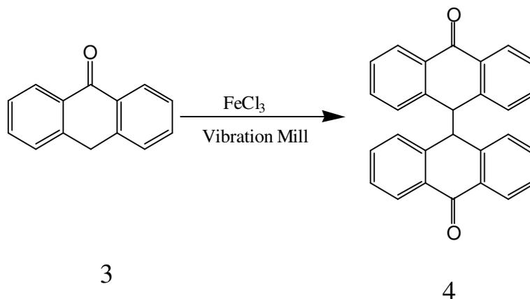
**Scheme 2.** Oxidative coupling of anthrone in a vibration mill at 30 Hz.
