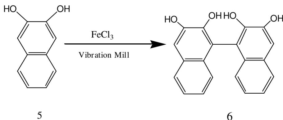
**Scheme 3.** Oxidative coupling of 2, 3-dihydroxy-1, 4-naphthylene in a vibration mill at 30 Hz.
