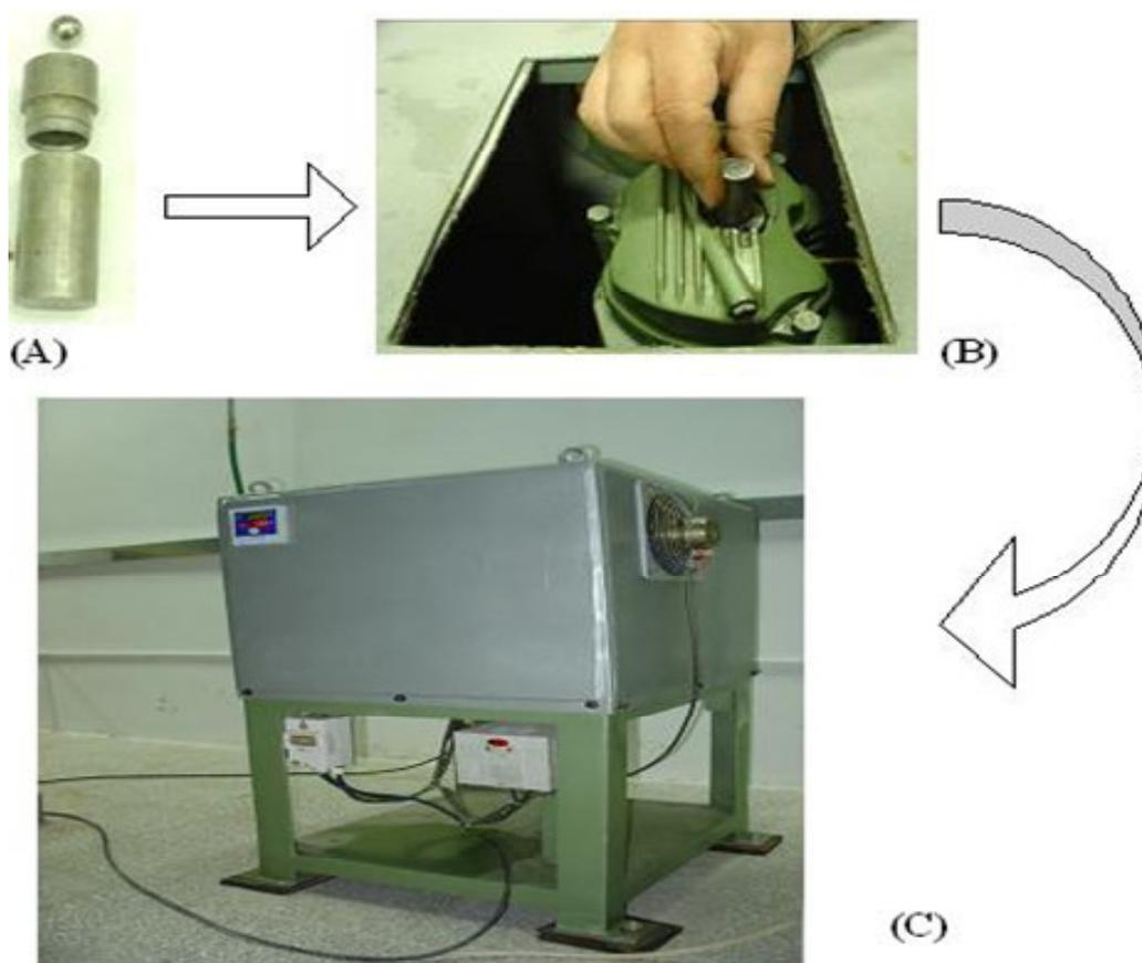
**Figure 1.** (a) Reaction chamber and ball, (b) Reactor holder, (c) Vibratory mill device.
