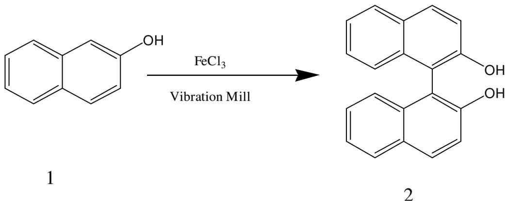
**Scheme 1.** Oxidative coupling of 2-Naphthol in a vibration mill.
