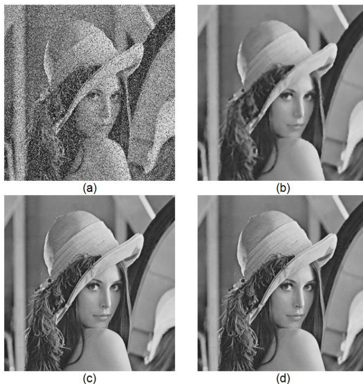
Figure 6. Image Lena corrupted by 25% of impulse noise (that is P = 0.25 ) (a), output from SM with size 7 \times 7 (b) and output from BDND using sorting operations (c) and output from BDND using local histograms (d).
