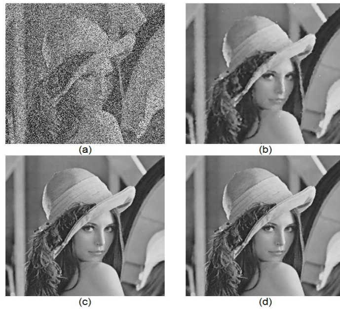
Figure 7. Image Lena corrupted by 50% of impulse noise (that is P = 0.50 ) (a), output from SM with size 7 \times 7 (b), output from BDND using sorting operations (c) and output from BDND using local histograms (d).
