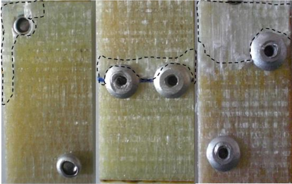
Figure 6. Failure states of riveted specimens.
