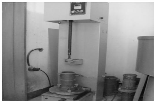
(a) Compaction test
