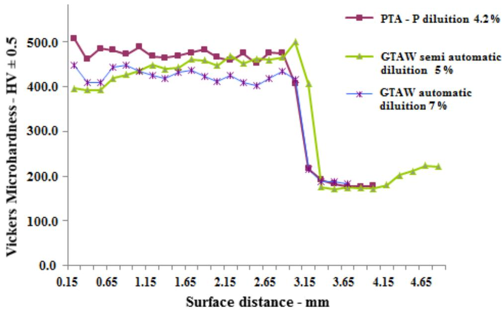
Figure 13. Micro hardness profiles for deposition of 19 g/min.
