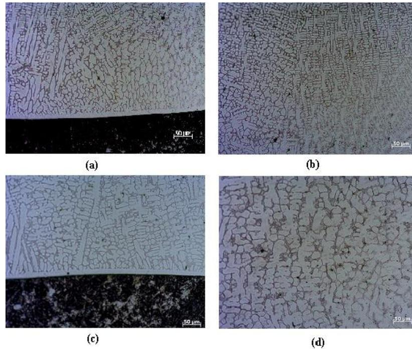
**Figure 3.** Micrographs of Powder Coating GTAW1 semi-automatic (a) close to the interface and (b) near the surface and GTAW2 (c) close to the interface d) near the surface.
