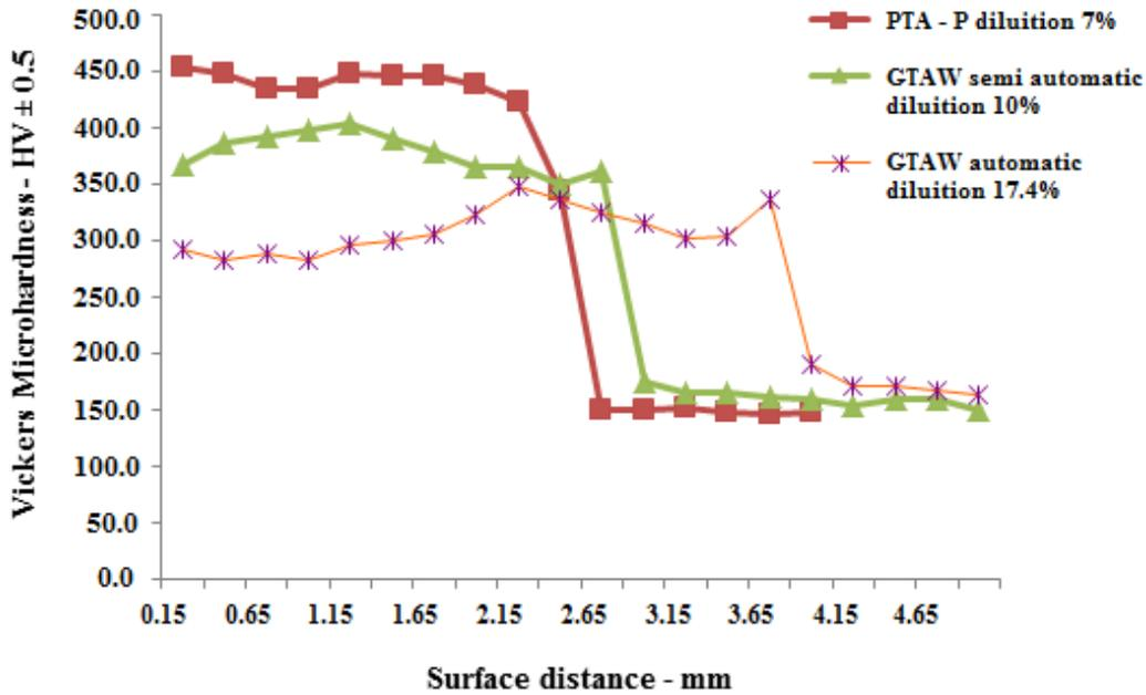
Figure 12. Micro hardness profiles for deposition of 9.5 g/min.
