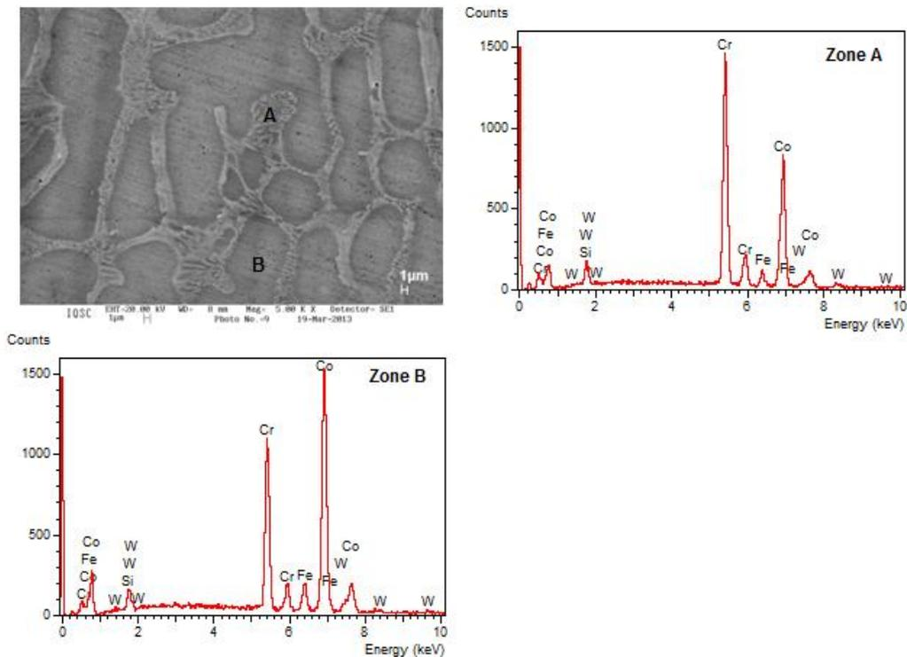
**Figure 8.** SEM of the coating GTAW2- semi-automatic close to the surface of the coating and its EDS zones A and B.
