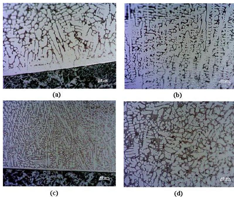
**Figure 4.** Micrographs of Coating PTA1 (a) close to the interface (b) close to the surface and PTA2 (c) close to the interface (d) near the surface.
