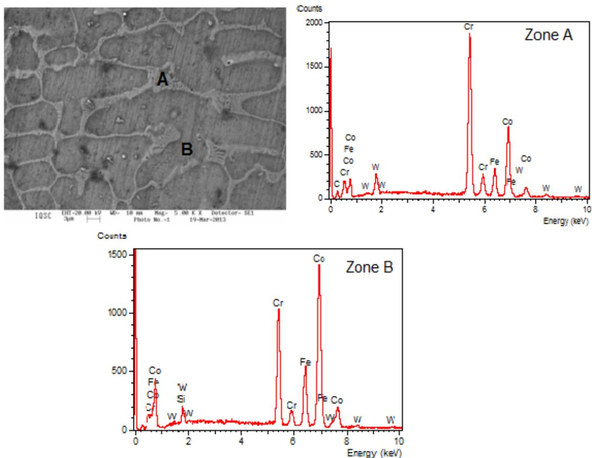
**Figure 5.** SEM of the coating GTAW1– automatic close to the surface of the coating and its EDS zones A and B.
