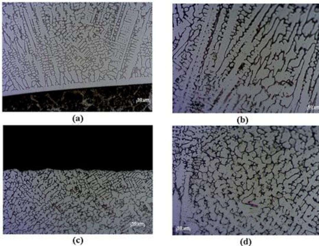
**Figure 2.** Micrographs of Powder Coating GTAW1 automatic (a) close to the interface and (b) near the surface and GTAW2 (c) close to the interface and (d) near the surface.
