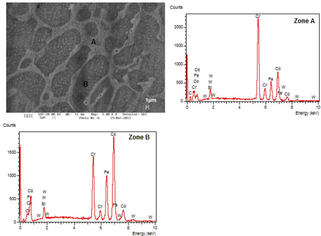
**Figure 7.** SEM of the coating GTAW1 semi-automatic close to the surface of the coating and its EDS zones A and B.
