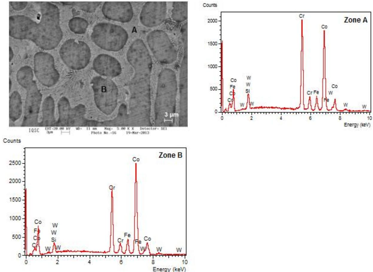
**Figure 10.** SEM of the coating PTA2- automatic close to the surface of the coating and its EDS zones A and B.
