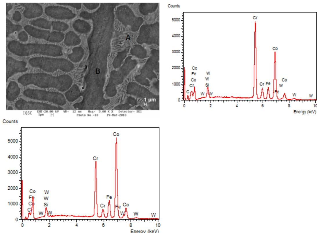
**Figure 9.** SEM of the coating PTA1- automatic close to the surface of the coating and its EDS zones A and B.
