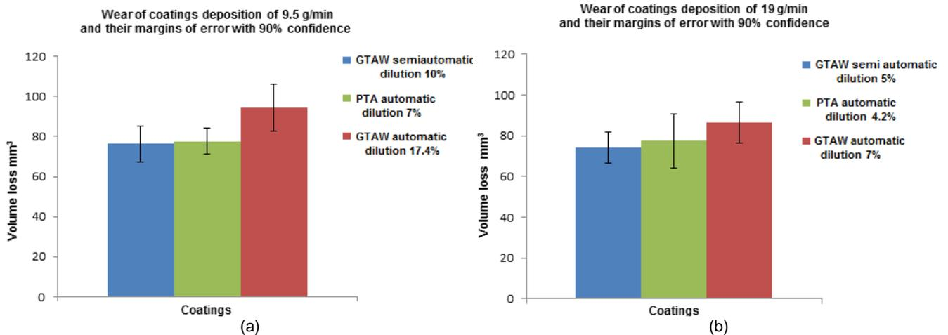
**Figure 11a.** Loss of volume wear test under the condition of deposition of (a) 9.5 and (b) 19 g/min, respectively.
