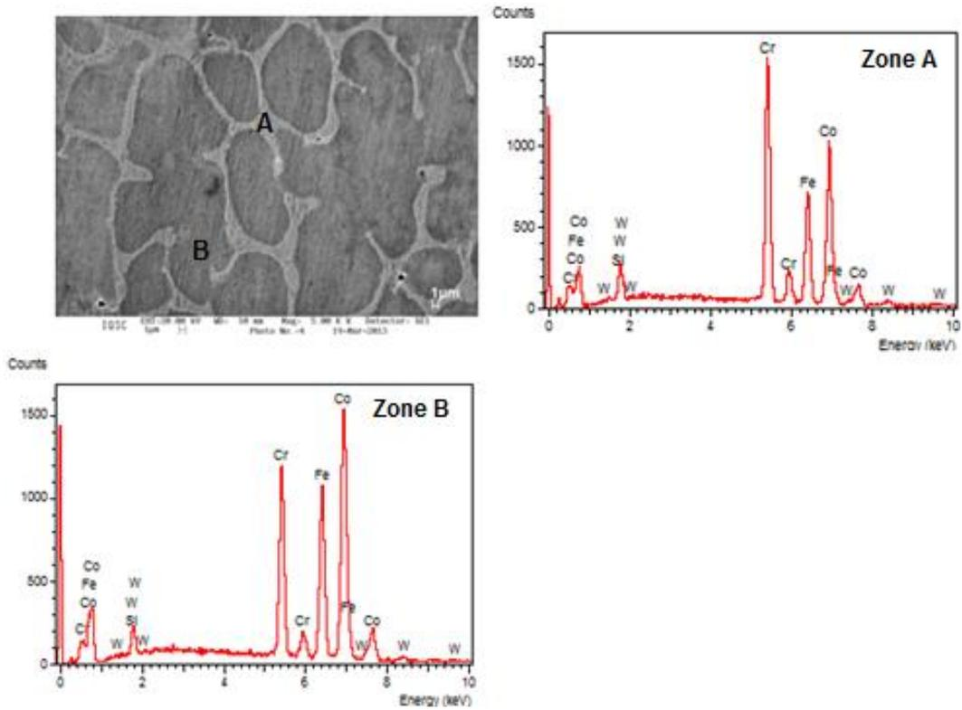
**Figure 6.** SEM of the coating GTAW2- automatic close to the surface of the coating and its EDS zones A and B.
