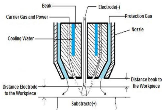
**Figure 1.** Device used for powder deposition by GTAW process - schematic representation.
