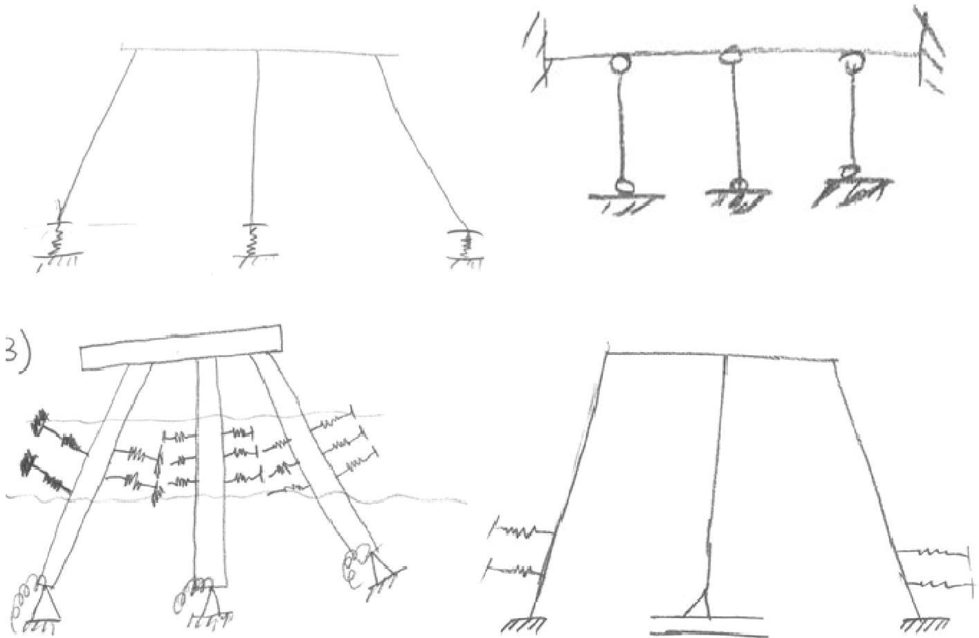
Figure 8. Example drawings with incorrect boundary conditions.
