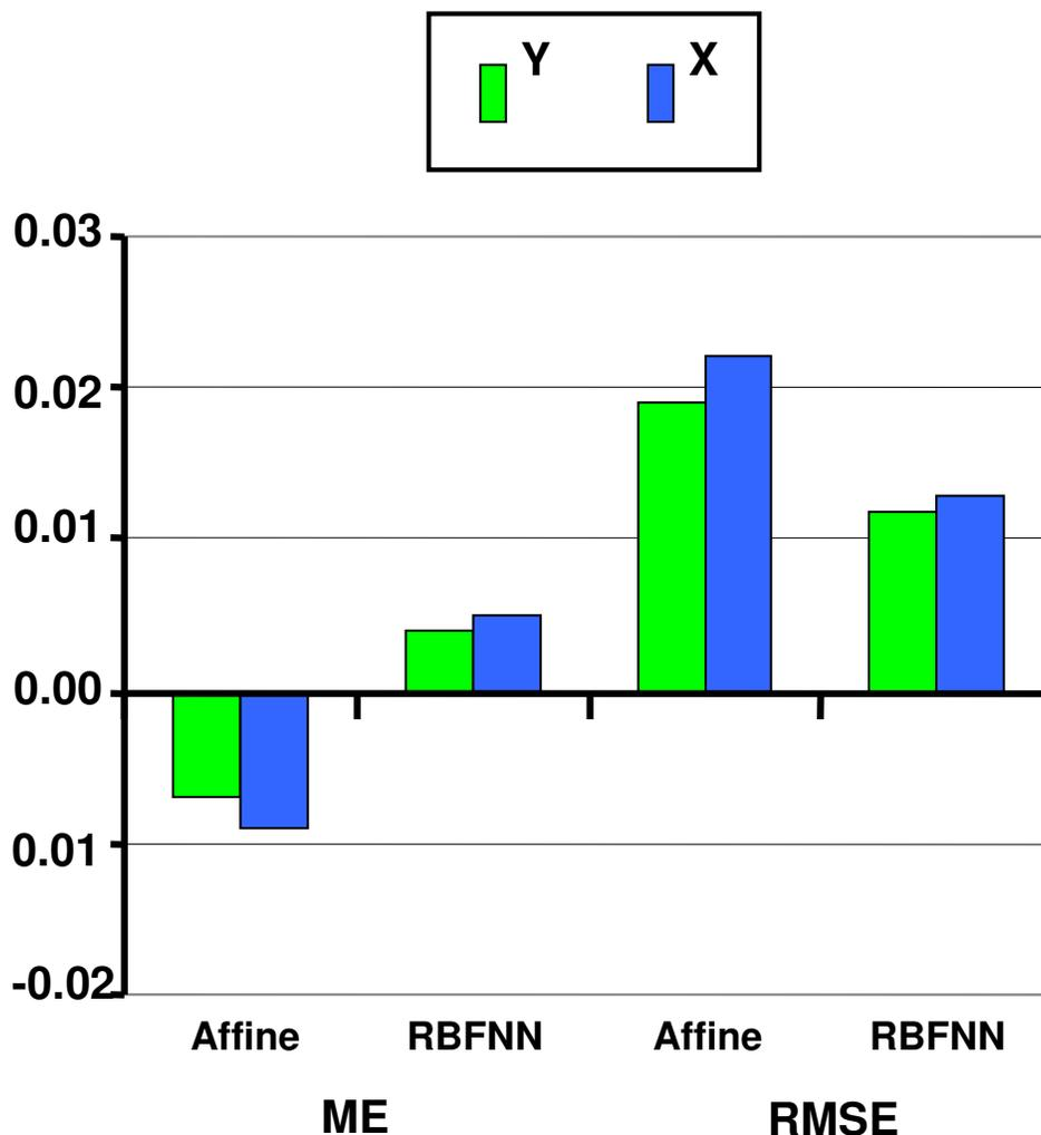
**Figure 3.** The check data set's ME and RMSE values based on Affine method and RBFNN (units in m).
