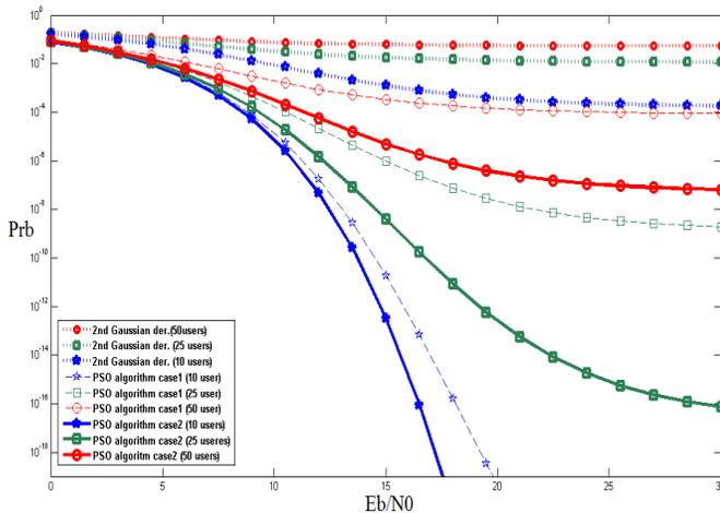
**Figure 9.** The  $Pr_b$  of PSO linear combined UWB pulse using  $e_1$ .
