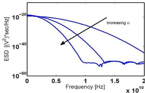
**Figure 2.** The Gaussian pulse changes with  $\alpha$  (Frequency domain).
