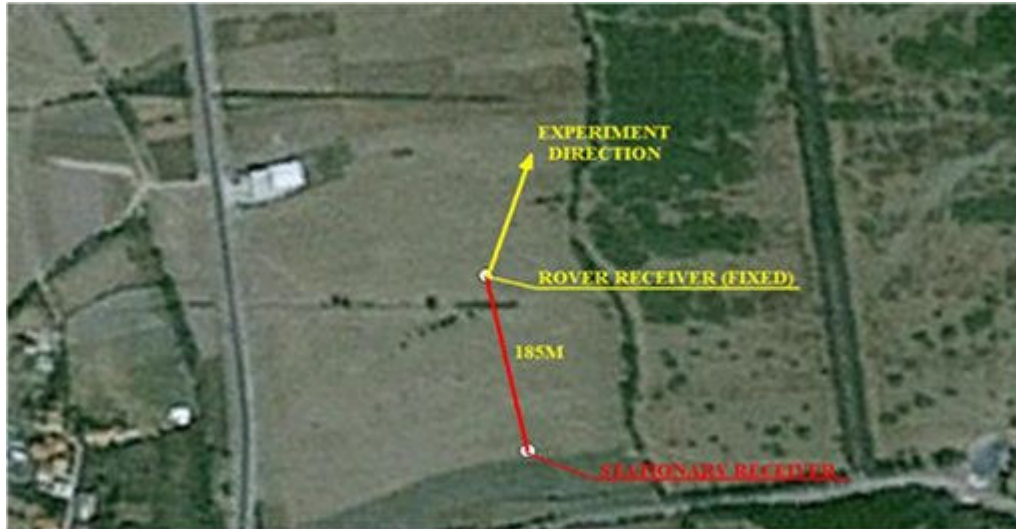
Figure 6. The experiment area and the locations of reference (stationary) and the test (rover) receivers (Courtesy of Google Earth™).
