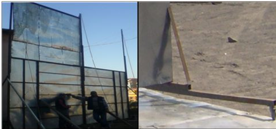
Figure 7. Vertical reflecting panel and its supporting bars and wheels.
