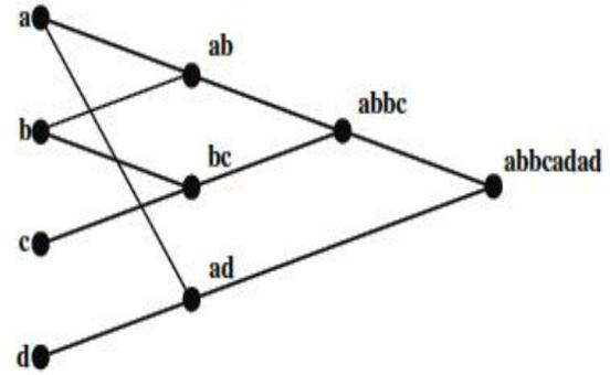
Figure 3. A generalized GMDH network structure of chromosome.
