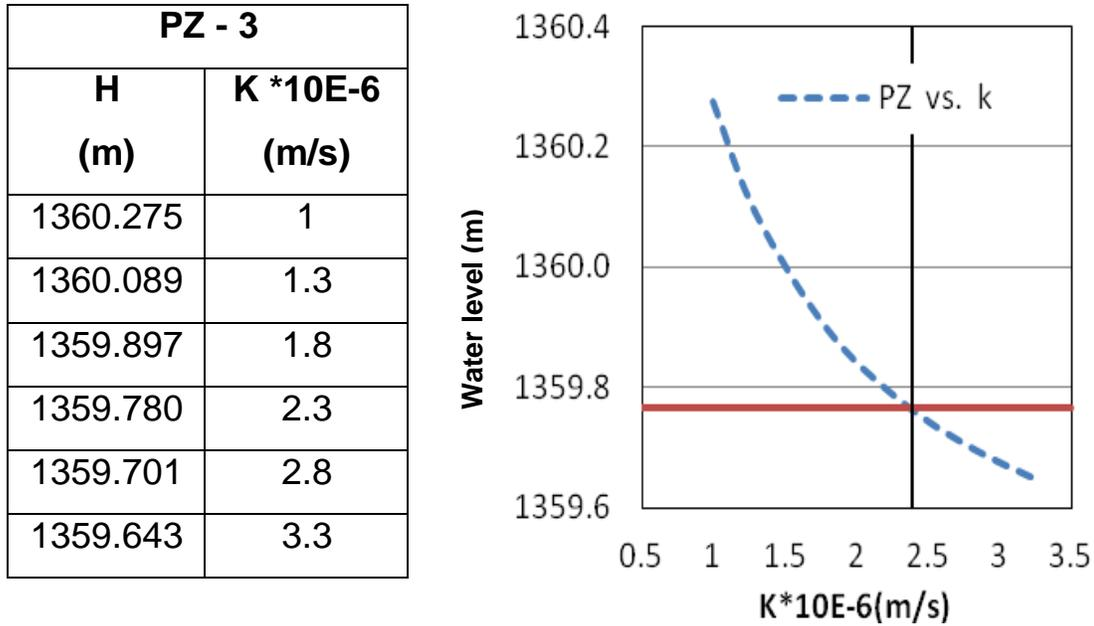
Figure 4. Back analyses of foundation permeability at critical section of dam.
