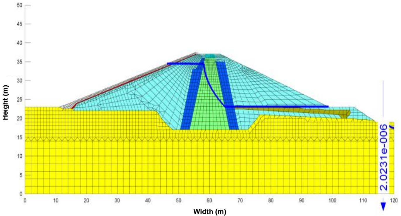
Figure 5. Seepage model in critical section by SEEP/W software.
