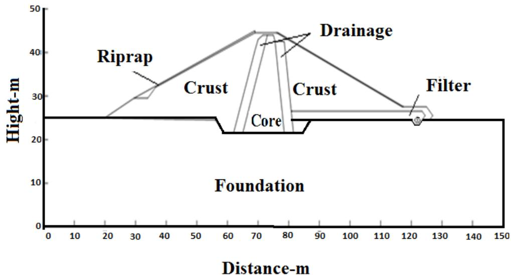
Figure 2. Cross section of FealehKhaseh earth Dam.
