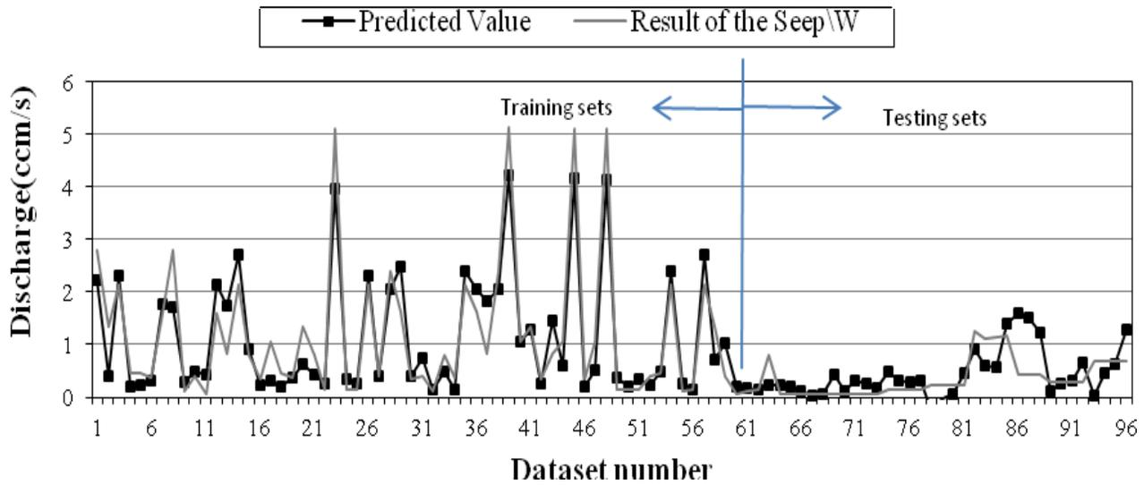
Figure 6. Neural network model predicted performance in comparison with SEEP\W predictions.
