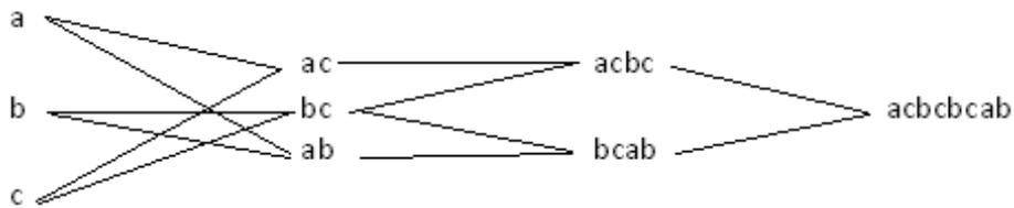
Figure 7. Evolved structure of GMDH neural network for prediction of seepage discharge.
