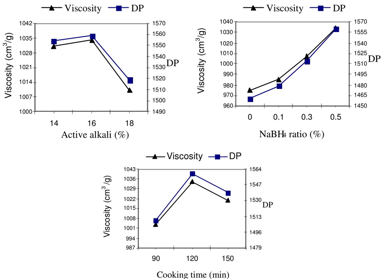
Figure 4. The effect of cooking conditions on viscosity (cm<sup>3</sup>/g) and DP.
