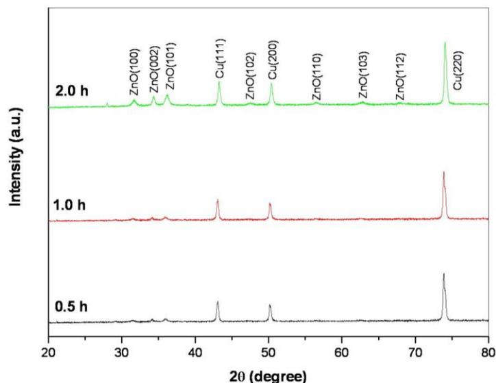
**Figure 3.** XRD patterns of cluster-assembled ZnO films on a copper substrate with various reaction times.
