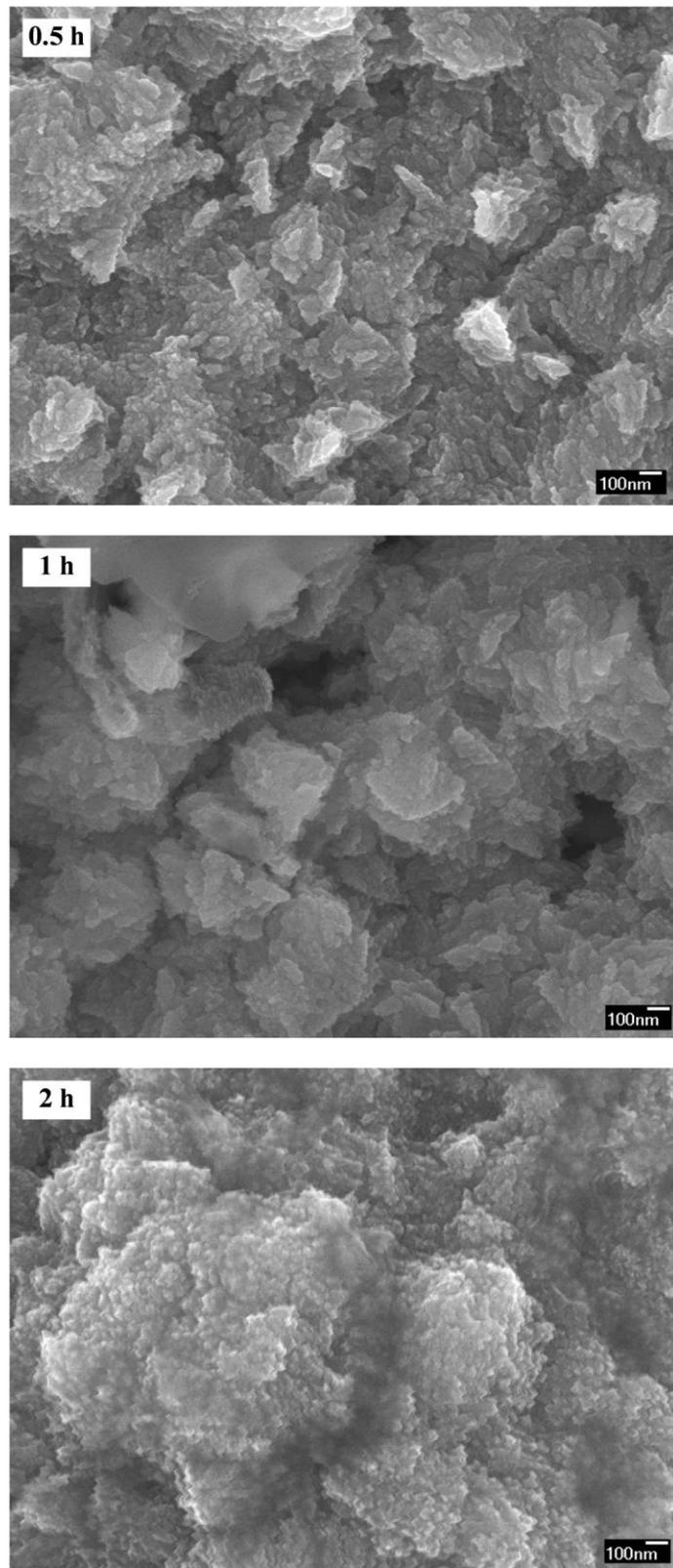
**Figure 1.** FE-SEM micrographs of cluster-assembled ZnO films on a copper substrate with various reaction times.
