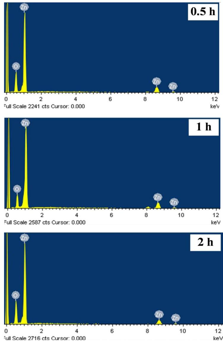
**Figure 2.** EDS spectra of cluster-assembled ZnO films on copper substrate with various reaction times.
