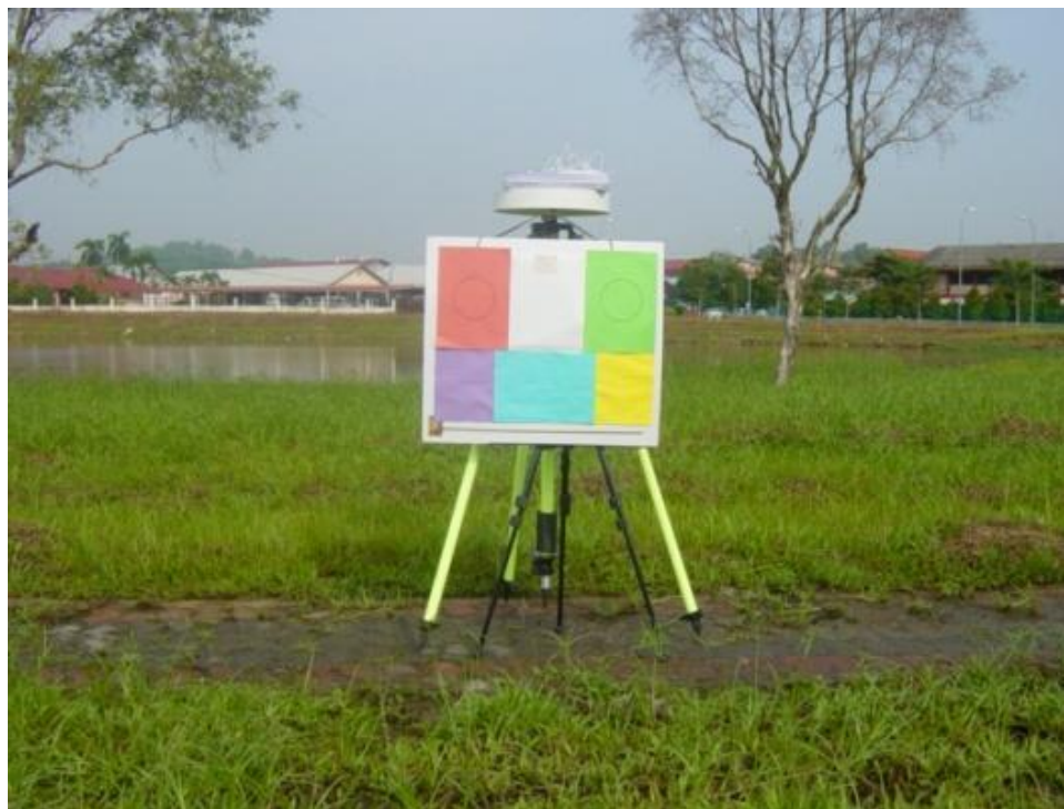
Figure 2. Apparatus used in building daylight color model with the white Munsell N/9 paper.
