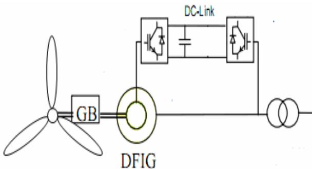
Figure 5. Double feed induction generator.
