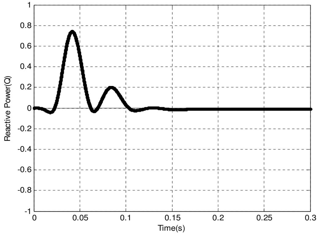
Figure 12. STATCOM reactive power controller.
