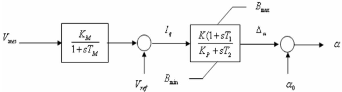
Figure 4. SVC voltage controller unit.
