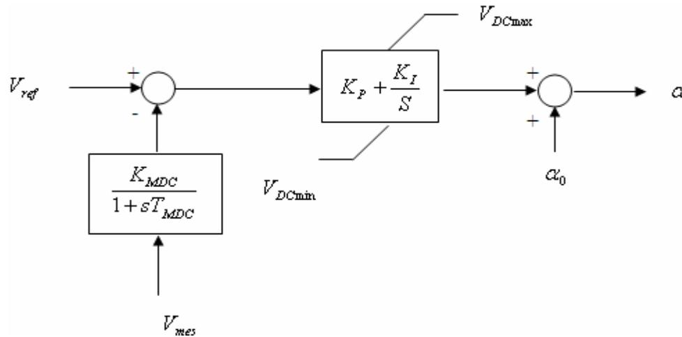
Figure 2. STATCOM voltage control unit.
