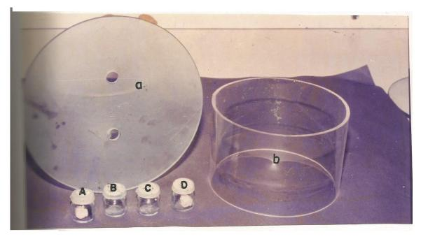
**Plate 2.** A Close-up of the olfactometer set-up used for the study of the banana weevil, C. sordidus pheromones in the laboratory. a= perforated basal glass plate of arena, b= the glass ring arena, A, B, C, D = glass containers for emitting weevils.
