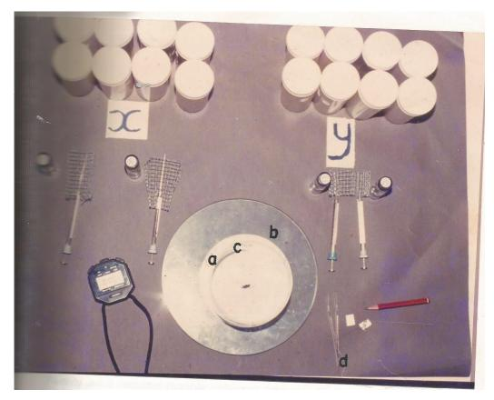
**Plate 1.** The experimental set-up for bioassaying extracts of the banana weevil, *C. sordidus* in the laboratory. x = responding weevils (males); y = responding weevils (females); a = the glass ring arena; b = the basal glass plate of the arena; c = filter paper placed underneath the arena; d = a pair of soft forceps.
