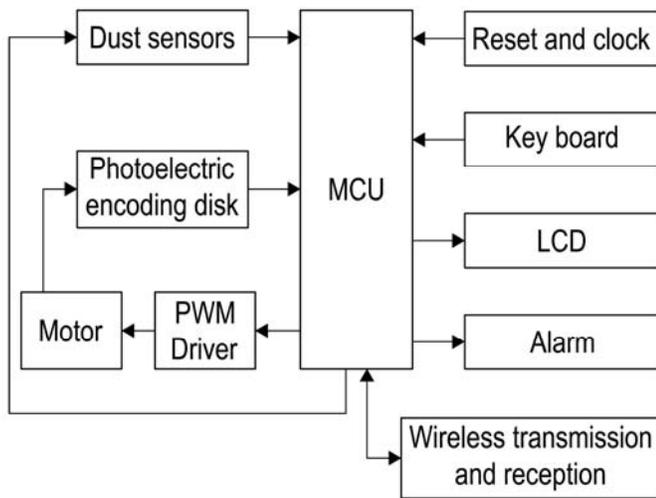
**Figure 1.** Structural diagram of the dust-concentration monitor.
