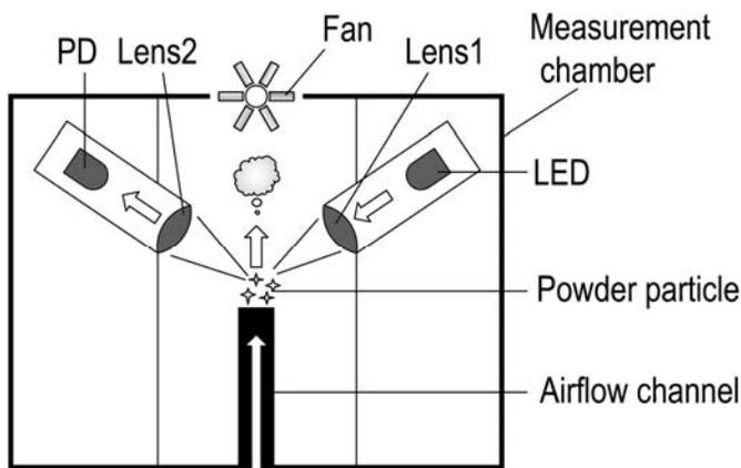
Figure 2. Structural diagram of dust sensor.
