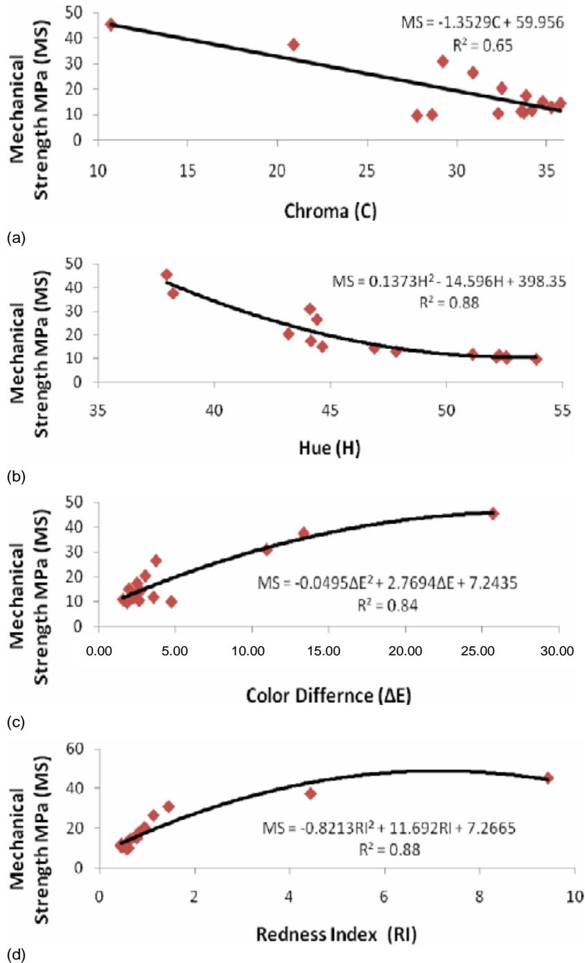
**Figure 2.** Relationships between mechanical strength (MS) and color parameters of clay bricks; (a) between mechanical strength (MS) and chroma; (b) between MS and hue; (c) between MS and color difference; (d) between MS and redness index.
