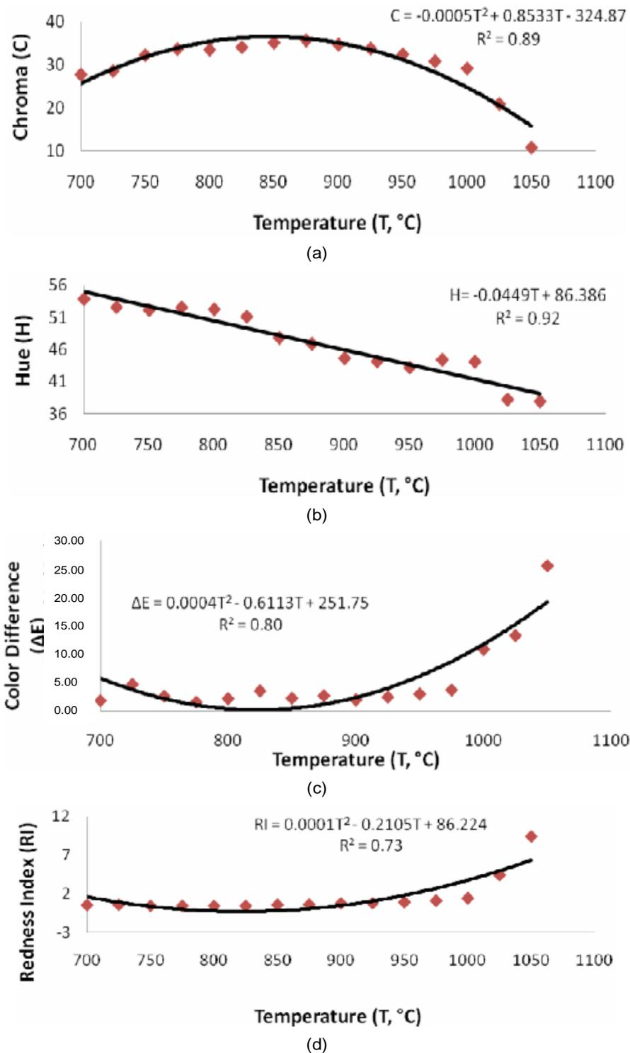
**Figure 1.** Relationships between firing temperature (FT) and color parameters of clay bricks; (a) between firing temperature; (FT) and chroma; (b) between FT and hue; (c) between FT and color difference; and (d) between FT and redness index.
