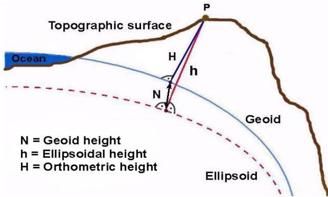
Figure 1. Geoid, ellipsoidal and orthometric heights.
