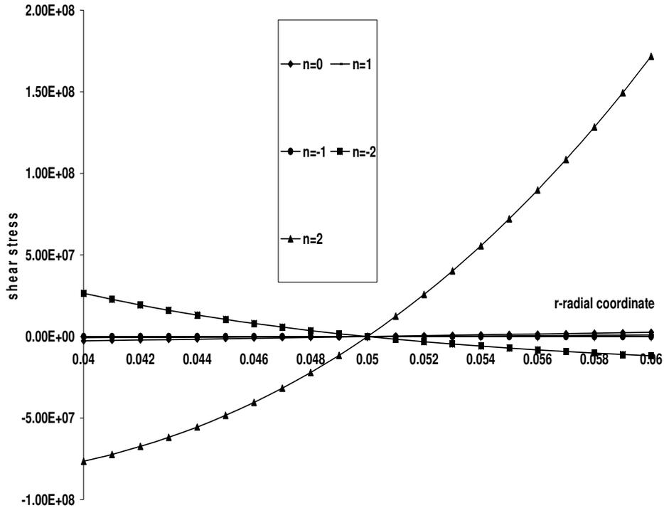
Figure 5. Distribution of shear stress in terms of n for 100°C temperature rising.
