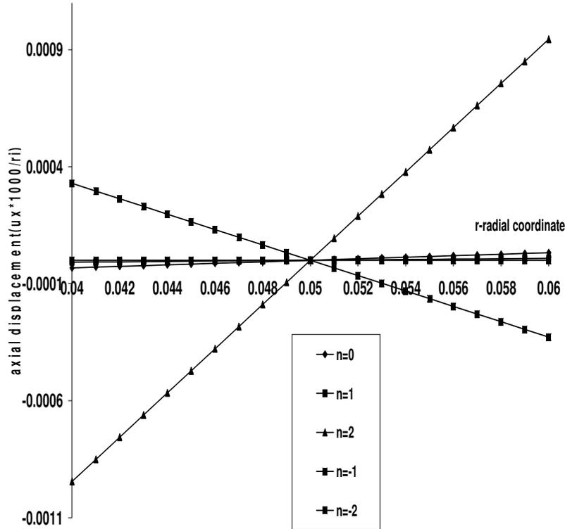
**Figure 4.** Axial displacement of FG cylinder under 100°C temperature rising in terms of *n*.
