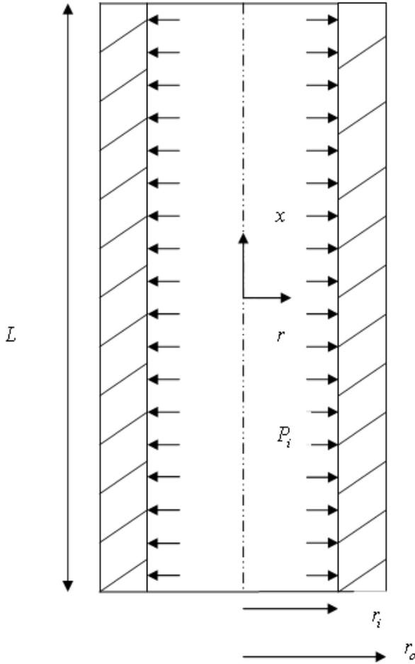
Figure 1. Schematic figure of cylindrical pressure vessel under applied inner and outer pressure.
