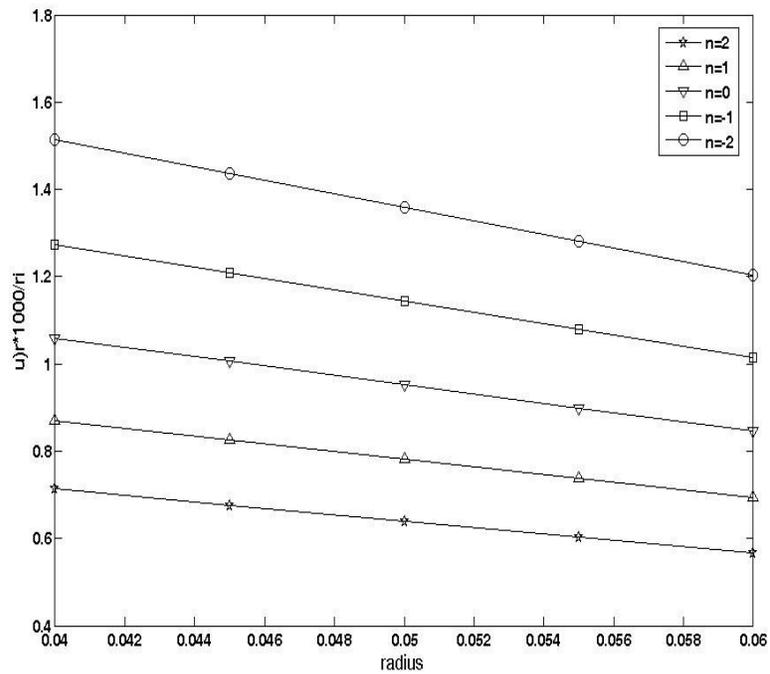
**Figure 8.** Radial distribution of displacement under only inner pressure (80 Mpa).
