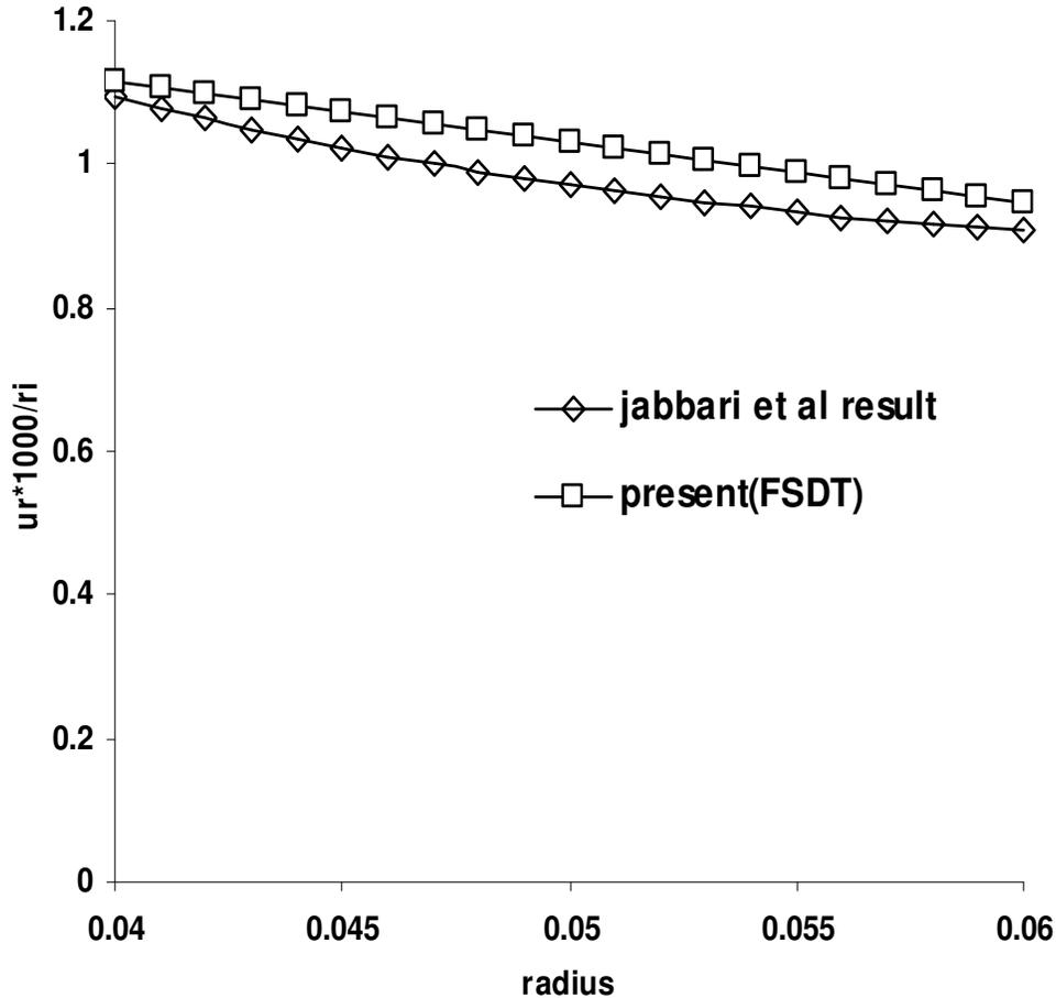
Figure 9. Comparing of the present result (FSDT) with result of plane elasticity theory (Jabbari et al).
