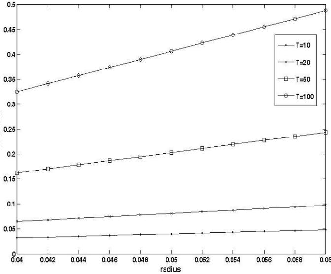
**Figure 2.** Radial displacement of FG cylinder with  $n=1$  and in terms of different temperature rising.
