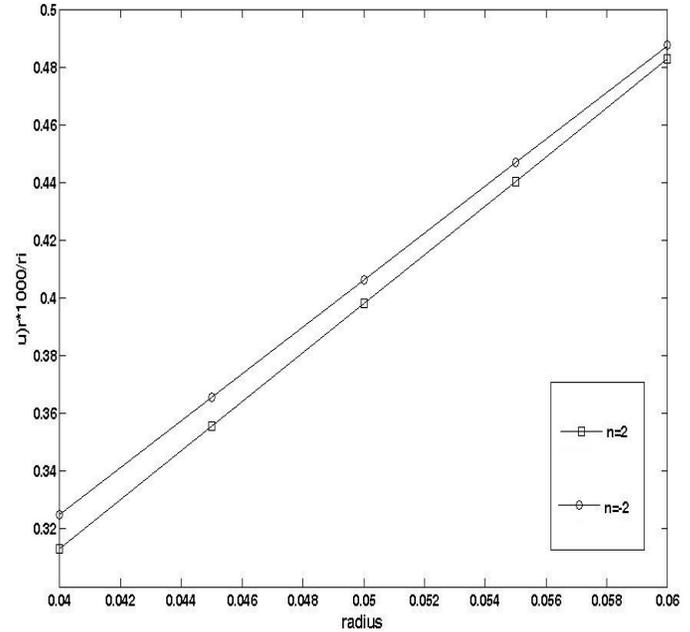
**Figure 3.** Comparison of radial displacement for 100°C. Temperature rising in terms of two non- homogenous coefficient of elasticity.
