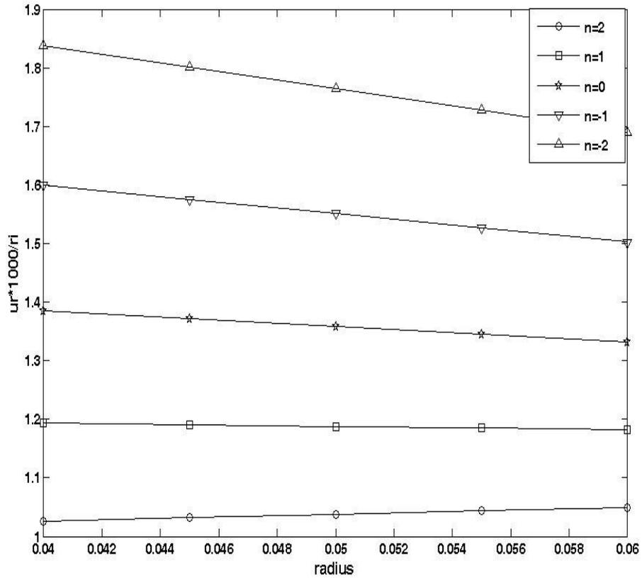
**Figure 7.** Distribution of radial displacement for 100 centigrade temperature rising and inner pressure 80 Mpa.
