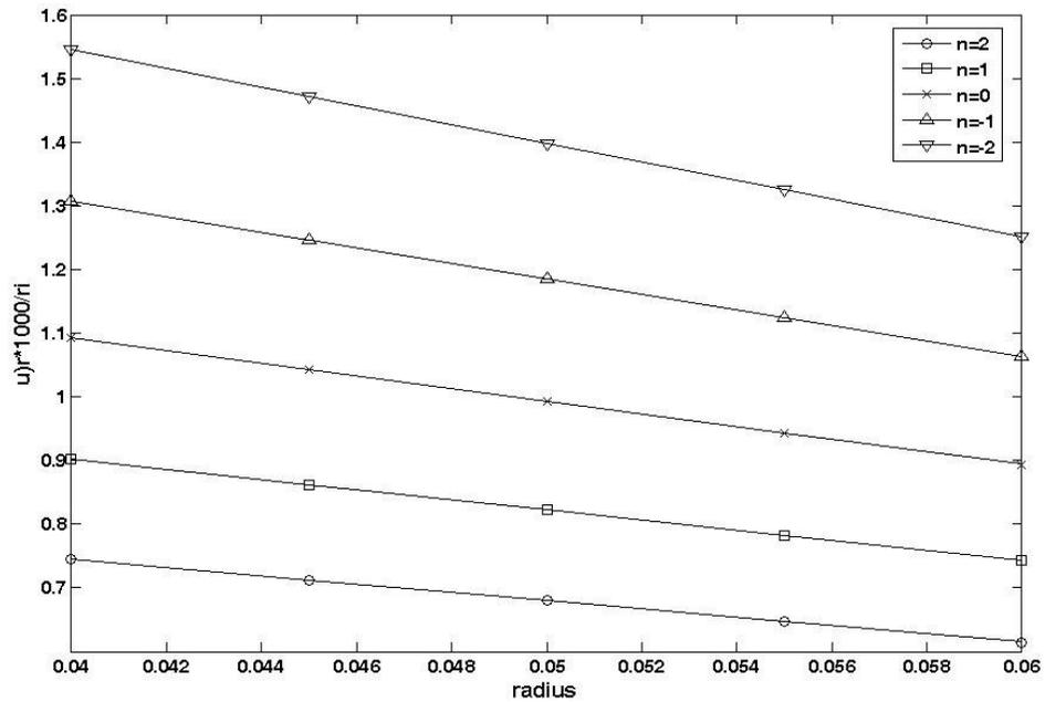
Figure 6. Distribution of radial displacement for 10°C temperature rising and inner pressure 80 Mpa.
