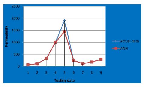
Figure 7. Comparison between graph produce of data permeability in lab and prediction by ANN in testing process.
