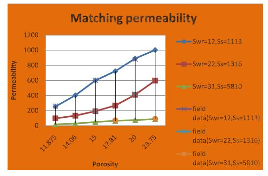
Figure 8. Matching field data with network data in testing process.
