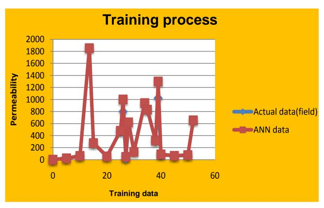
Figure 6. Comparison between graph produce of data permeability in lab and prediction by ANN in training process.
