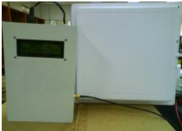
Figure 1. In house built in EPC Class 1 Gen 2 Passive RFID reader and antenna.
