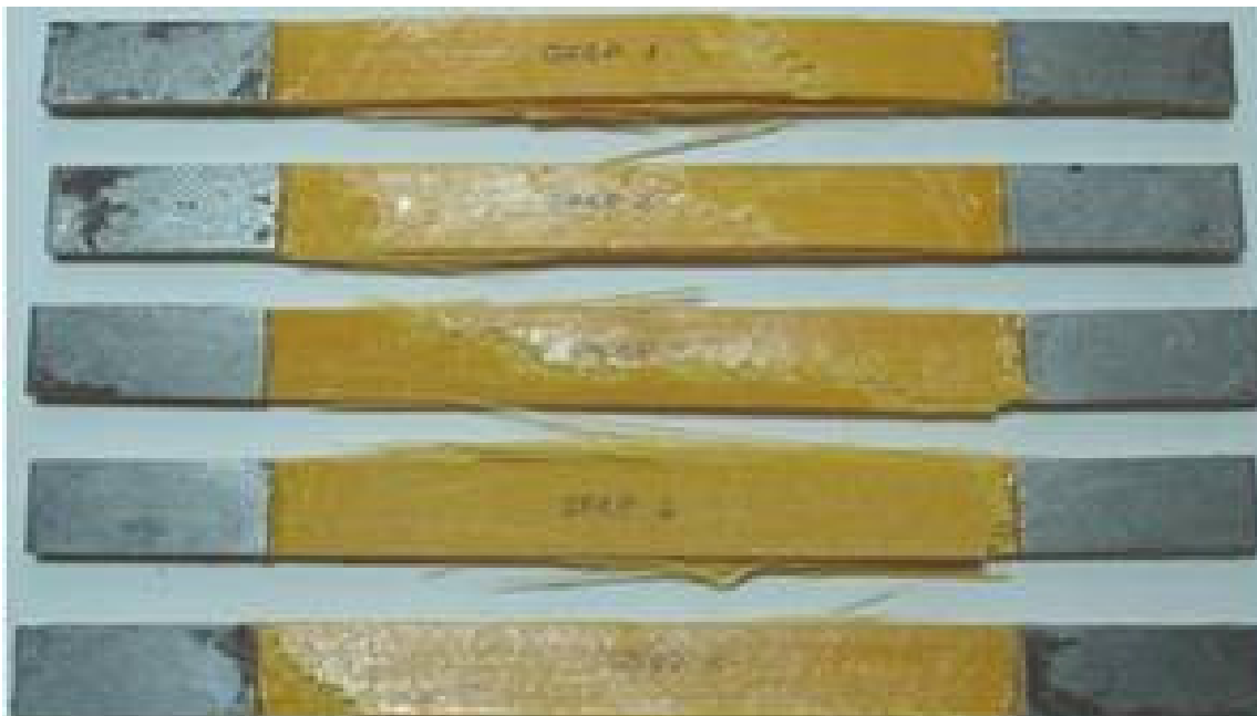
Figure 5. Pultruded GFRP tensile coupons with bonded steel tabs and failure modes.
